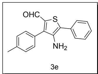
Yellow solid; mp: 125 – 126°C; <sup>1</sup>H NMR (500 MHz, CDCl<sub>3</sub>) δ 9.61(s, 1H), 7.63 (d, J = 7.15Hz, 2H), 7.46 (t, J = 7.51Hz, 2H), 7.38 – 7.32 (m, 5H), 3.79(s, 2H), 2.44(s, 3H); <sup>13</sup>C NMR (125 MHz, CDCl<sub>3</sub>) δ 184.10, 142.50, 140.52, 139.17, 136.49, 133.51, 130.02, 129.82, 129.90, 129.42, 128.22, 128.09, 125.94, 21.44; HRMS (ESI): m/z calcd for C<sub>18</sub>H<sub>15</sub>NOS [M+H]<sup>+</sup>: 294.0953, found: 294.0949.
