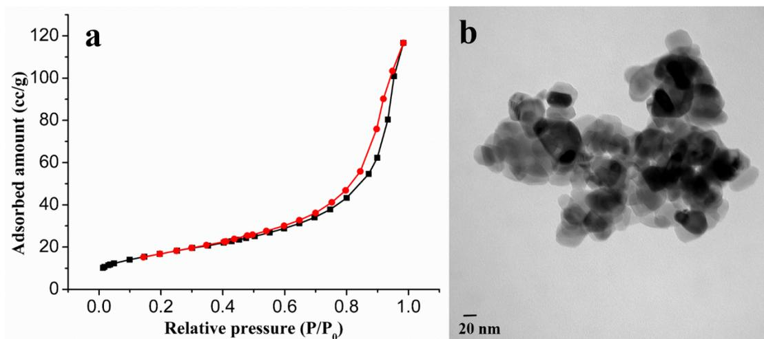
**Fig. S8** The adsorption-desorption isotherms and TEM image of commercial  $\text{TiO}_2$ .
