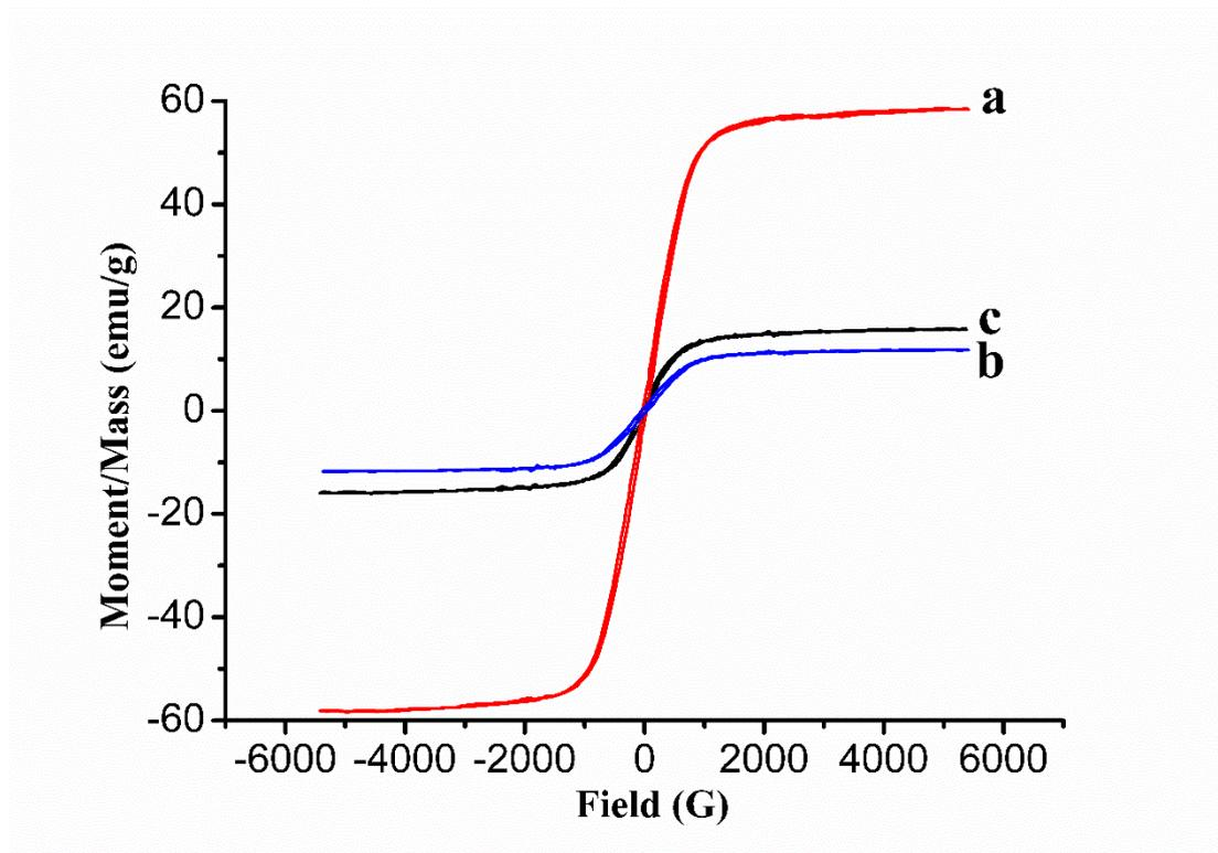
**Fig. S3** Room-temperature magnetization curve of (a)  $\text{Fe}_3\text{O}_4$ , (b)  $\text{Fe}_3\text{O}_4@m\text{TiO}_2@m\text{SiO}_2\text{-CTAB}$  and (c) YS  $\text{Fe}_3\text{O}_4@m\text{TiO}_2@m\text{SiO}_2$ .
