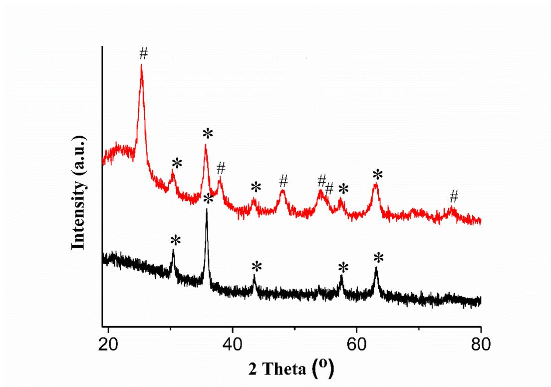
**Fig. S1** XRD spectrum of Fe<sub>3</sub>O<sub>4</sub> (black line) and YS Fe<sub>3</sub>O<sub>4</sub>@mTiO<sub>2</sub>@mSiO<sub>2</sub> (red line). \* and # indicate the diffraction peaks of magnetite phase of Fe<sub>3</sub>O<sub>4</sub> and anatase TiO<sub>2</sub>, respectively.
