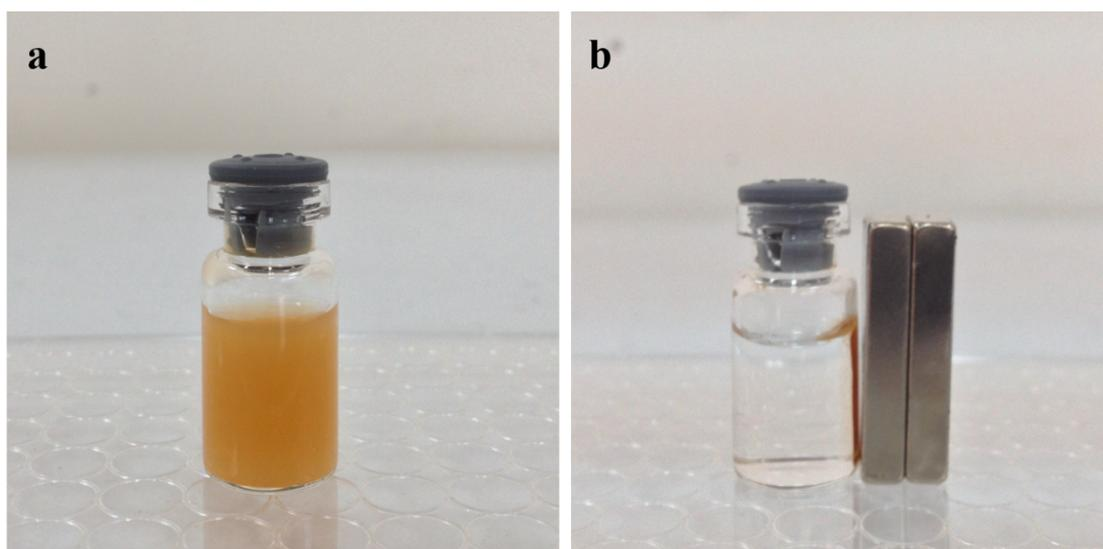
**Fig. S7** The images of a water dispersion of YS  $\text{Fe}_3\text{O}_4@m\text{TiO}_2@m\text{SiO}_2$  (a) before and (b) after magnetic separation.
