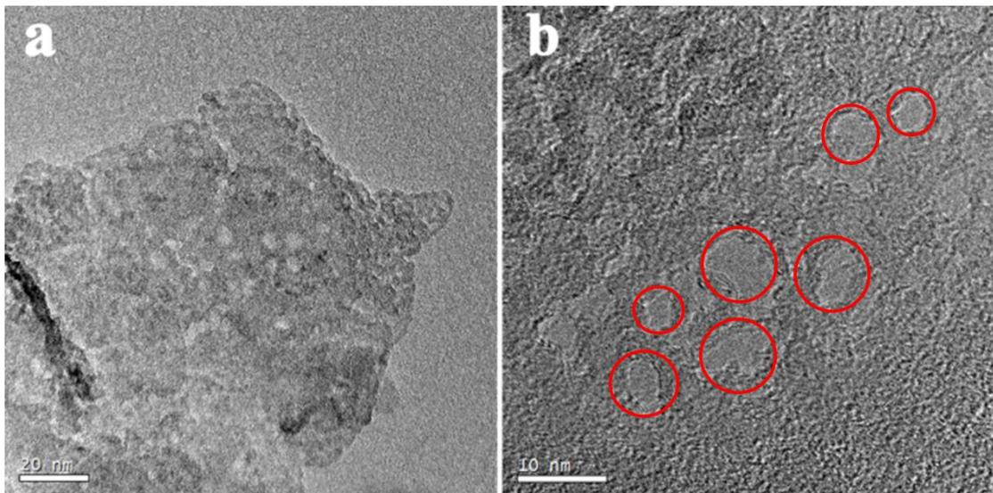
Figure S3. (a) (b) TEM images of the composite show a highly random porous architecture of the nanosheets
