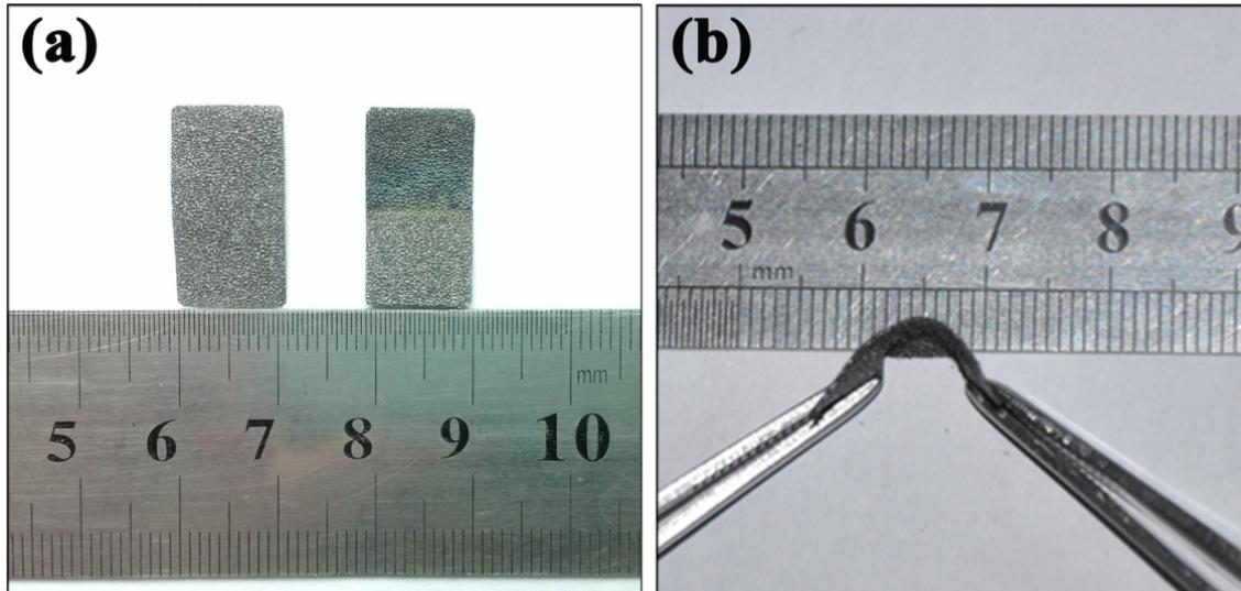
Figure S2. (a) The photo images of the pristine 3DG (left) and the Ni(OH)<sub>2</sub> nanosheets/3D graphene composite (right), and (b) the flexible electrode.
