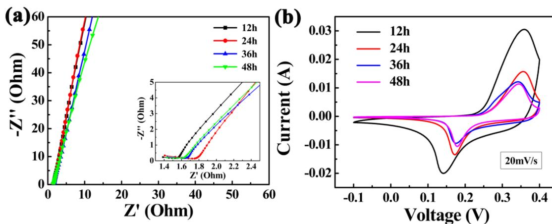
Figure S5. (a) Nyquist plots and (b) CV curves at the scan rates of  $20\text{ mV s}^{-1}$  of the  $\text{Ni}(\text{OH})_2$  nanosheets/3DG
