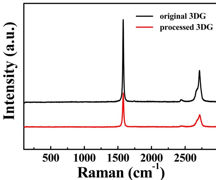
Figure S4. The Raman spectra of original 3DG and processed 3DG.
