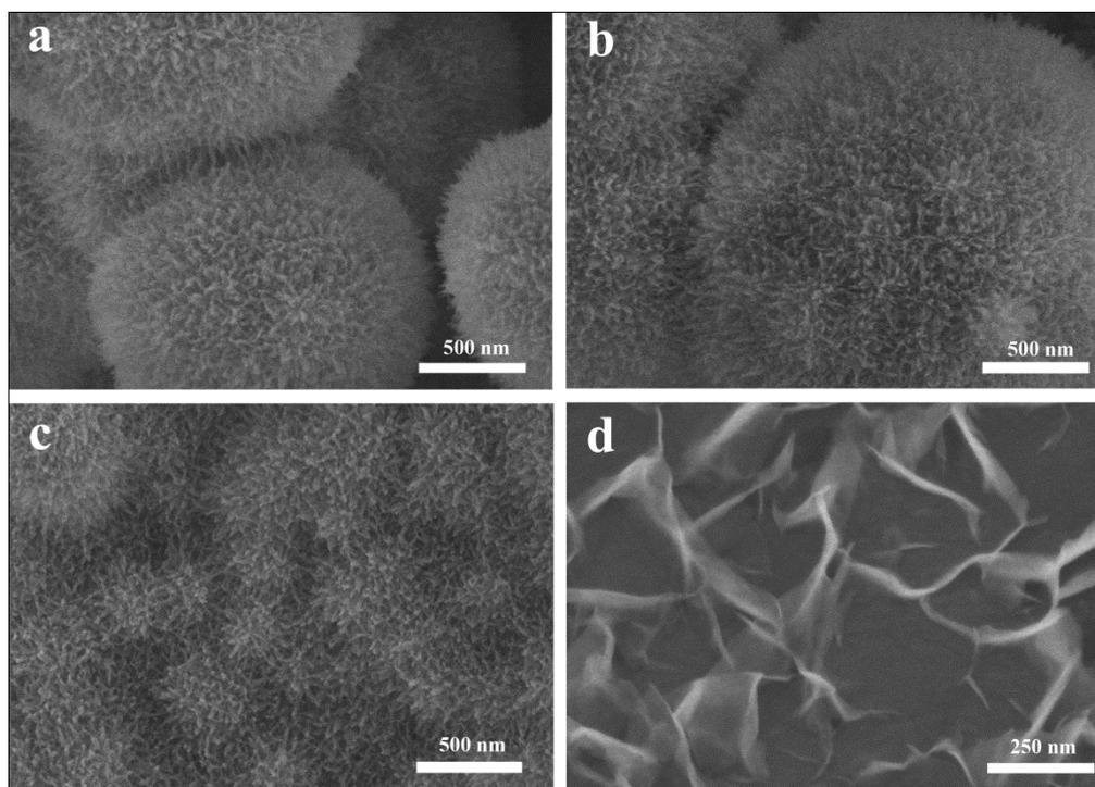
Figure S1. (a) (b) (c) (d) SEM images of the Ni(OH)<sub>2</sub> nanosheets/3D graphene composite made at 90 °C for 48, 36, 24, 12 h, respectively.
