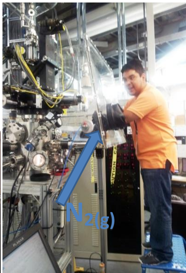
Fig S3. Inert (a) micro-Raman and (b) synchrotron based soft X-ray absorption spectroscopy experimental sample analysis set up.
