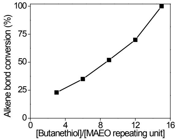
**Fig. S7.** Alkene bond conversion versus ratios of [butanethiol]/[MAEO repeating unit] plot for PMAEO reacting with butanethiol at a constant [MAEO repeating unit]/[AIBN] = 1:1 in THF at 60 °C (reaction time = 12 h). Conversion values were calculated by  $^1\text{H}$  NMR spectroscopy based on the consumption of the alkene bonds.
