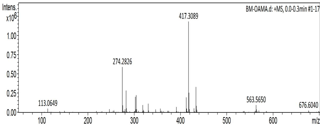
**Fig. S2** ESI-MS spectrum of MAEO (calculated  $m/z$  for  $[M + Na^+]$ : 417.308 and observed: 417.309).
