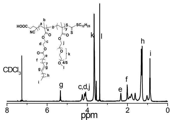
**Fig. S6** <sup>1</sup>H NMR spectra of PMAEO-*b*-PPEGMA.
