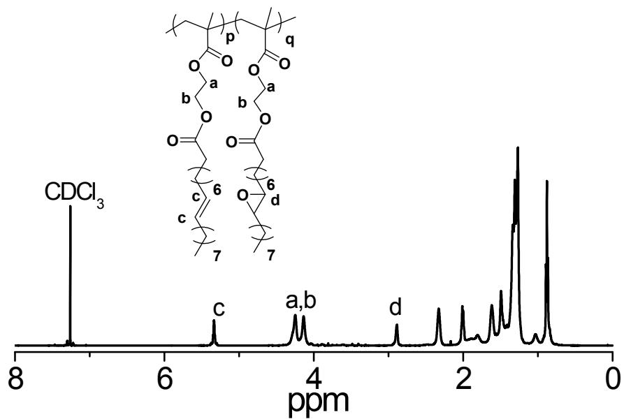
**Fig. S9**  $^1\text{H}$  NMR spectrum of epoxide of PMAEO obtained from the reaction at [MAEO repeating unit]/[mCPBA] = 2:1 ratio.
