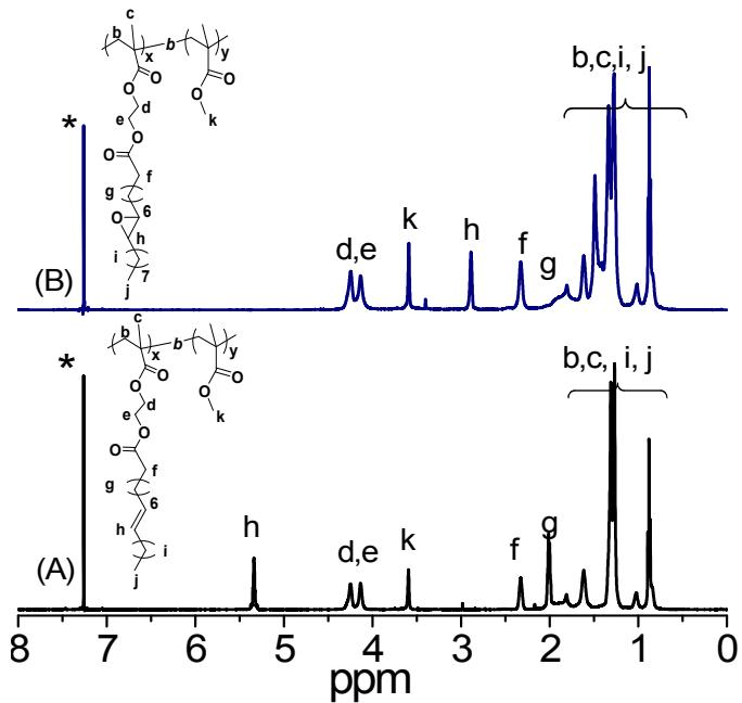
**Fig. S5** <sup>1</sup>H NMR spectra of PMAEO-*b*-PMMA (A) and PMAEO-*b*-PMMA in epoxide form (B).
