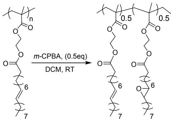
**Scheme S1** Post-polymerization modifications of the double bonds in PMAEO *via* epoxidation reaction at [MAEO repeating unit]/[mCPBA] = 2:1 ratio.
