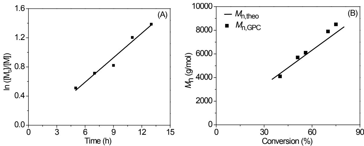
**Fig. S3** First-order kinetic plot for the RAFT polymerization of MAEO (A) and the corresponding  $M_n$  versus monomer conversion plot (B). Polymerization reaction was carried out at [MAEO]/[CDP]/[AIBN] = 25:1:0.2 in THF at 60 °C.
