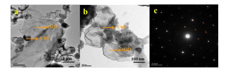
Fig. S1 High resolution TEM images of (a) CuS/rGO-x composites and (b) SAED pattern
