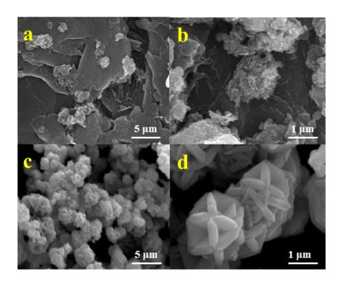
Fig. S2 High resolution SEM images of CuS/rGO-x composites (a-b) and pure CuS (c-d).
