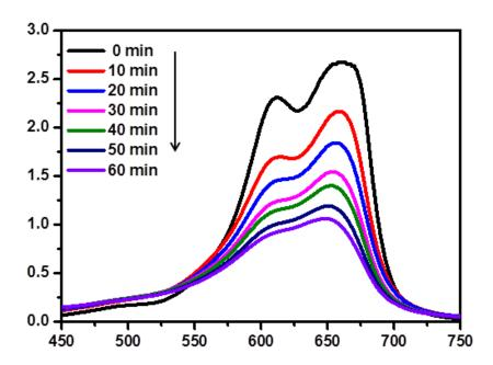
**Fig. S3** Photodecolourization of CuS/rGO composite by stirrer mixing for methylene blue dye under visible light irradiation.
