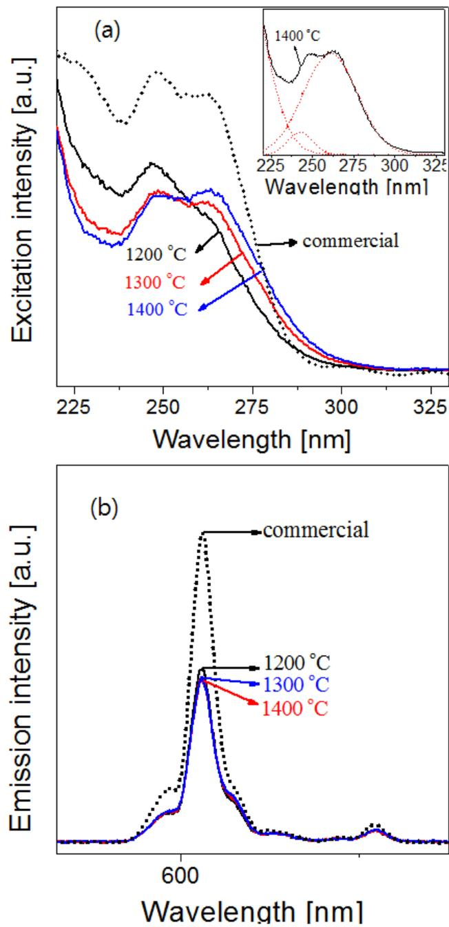
**Figure S6.** Excitation and emission spectra of the  $\text{Y}_2\text{O}_3:\text{Eu}^{3+}$  phosphor powders prepared by spray drying method and the commercial  $\text{Y}_2\text{O}_3:\text{Eu}^{3+}$  product.
