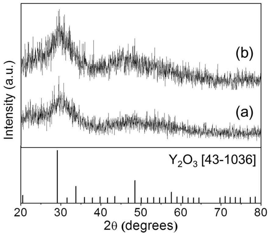
**Figure S7.** XRD patterns of the (a) first spray dried, and (b) crushed  $\text{Y}_2\text{O}_3:\text{Eu}^{3+}$  phosphor powders.
