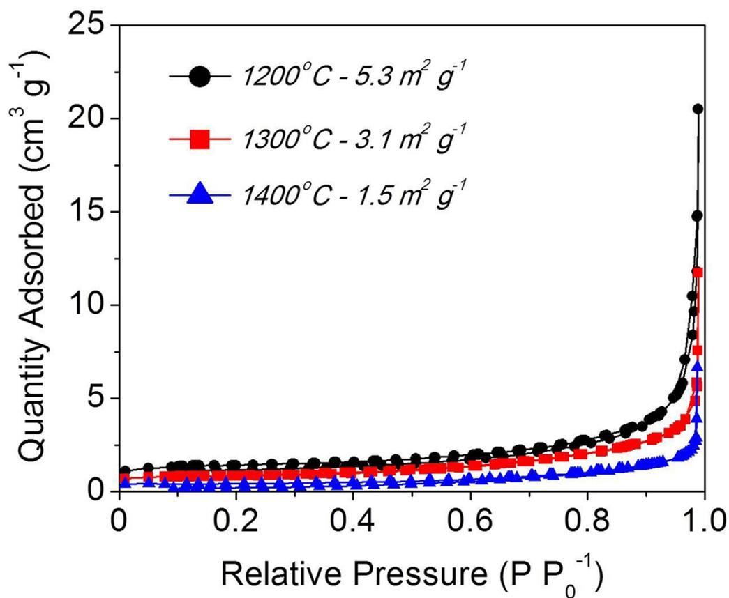
**Figure S4.** N<sub>2</sub> adsorption-desorption isotherms measured at 77 K for the Y<sub>2</sub>O<sub>3</sub>:Eu<sup>3+</sup> phosphor powders formed at the various sintering temperatures.
