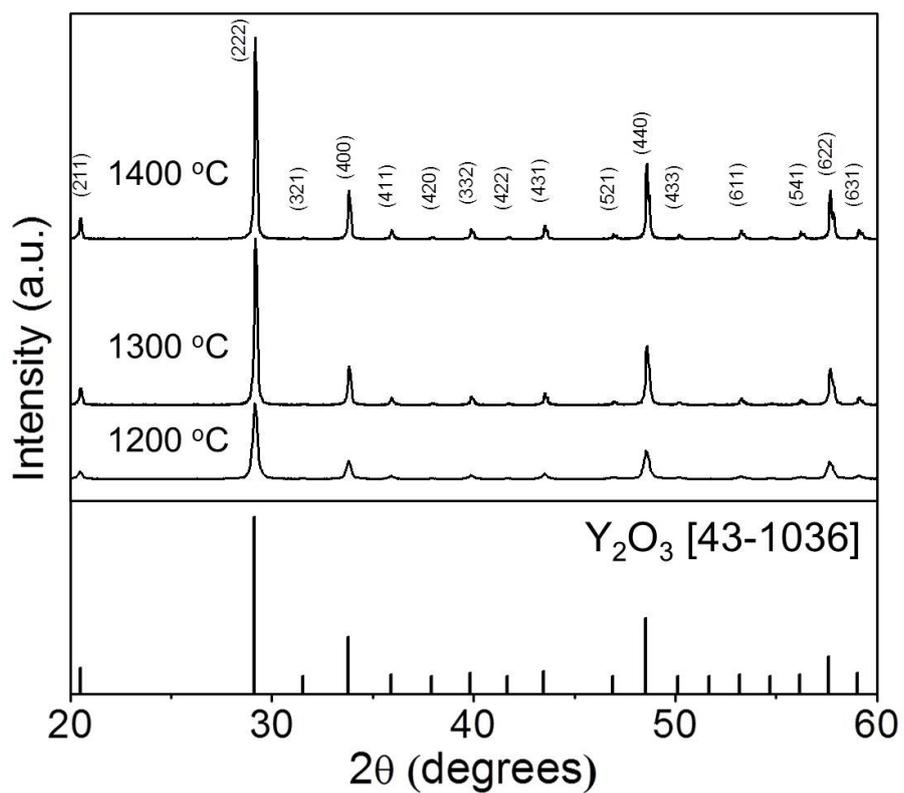
**Figure S5.** XRD patterns of the  $\text{Y}_2\text{O}_3:\text{Eu}^{3+}$  phosphor powders formed at the various sintering temperatures.
