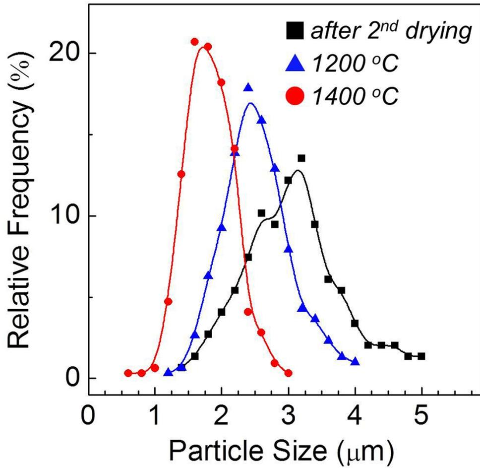
**Figure S3.** Particle size distributions of the  $\text{Y}_2\text{O}_3:\text{Eu}^{3+}$  phosphor powders before and after sintering process.
