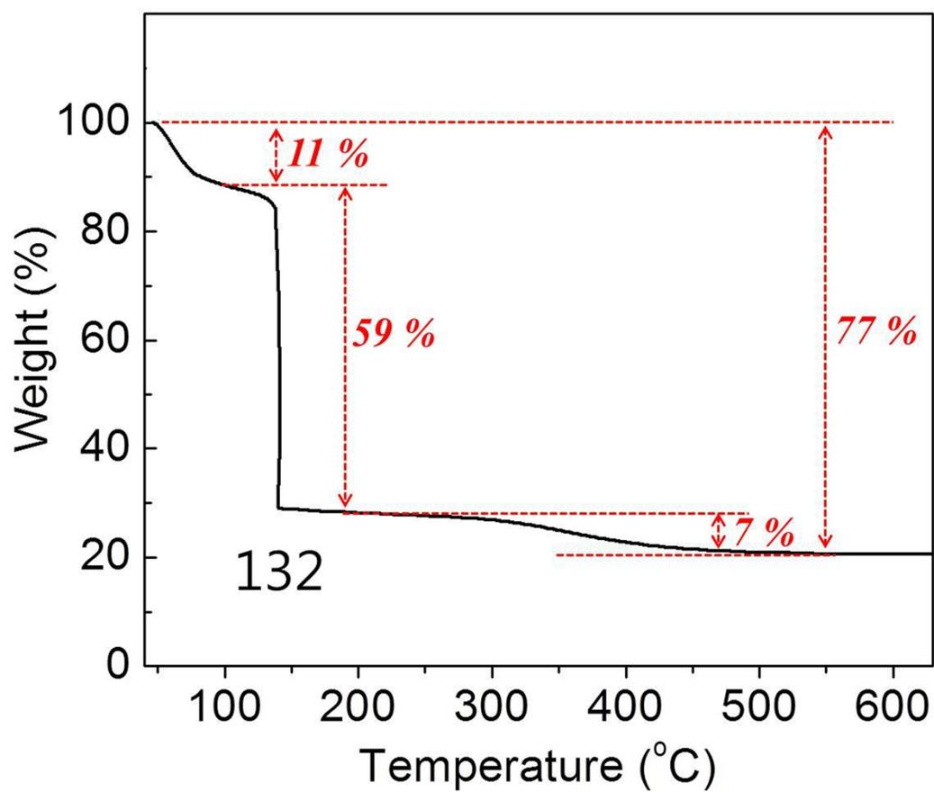
**Figure S2.** TG analysis of the Y<sub>2</sub>O<sub>3</sub>:Eu<sup>3+</sup> precursor powders directly prepared by first-step spray drying.
