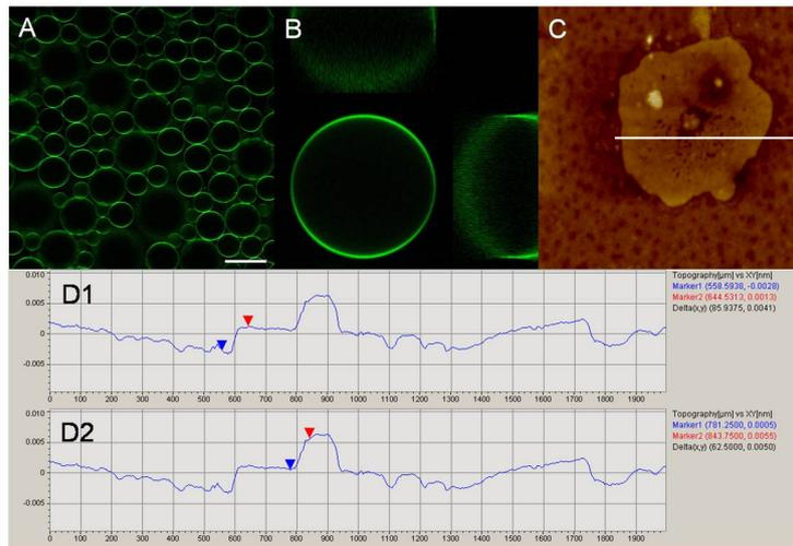
**Fig. S6** Images of the crosslinked capsules of MCoTI-II. (A) Fluorescent image investigated with LSCM with MCTI-I 0.1 mg/mL concentration; (B) Fluorescent image of LSCM in orthotic model; (C) Topography image investigated with AFM after totally dried with MCTI-I 1.0 mg/mL concentration; D1 and D2, Height analysis of the capsule in C. Scale bar is 200  $\mu\text{m}$  for A. The width of C is equal to 2  $\mu\text{m}$ .
