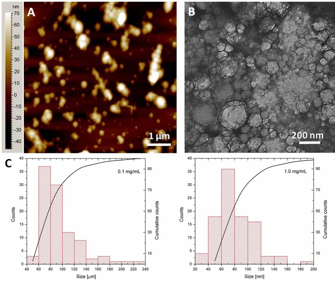
**Fig. S5** (A) AFM image of crosslinked capsules after dried 3 hours with MCTI-I 1.0 mg/mL concentration., (B) TEM image of crosslinked capsules with MCTI-I 1.0 mg/mL concentration, (C) Distribution of size measured for crosslinked droplets prepared with MCTI-I in 0.1 mg/mL and 1.0 mg/mL concentrations.
