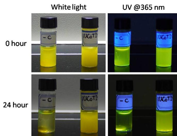
**Fig. S7** Optical images and fluorescence of emulsion prepared at 1.0 mg/mL of MCoTI-II pH 7.8 loading coumarine-6 and control mixture without MCoTI-II
