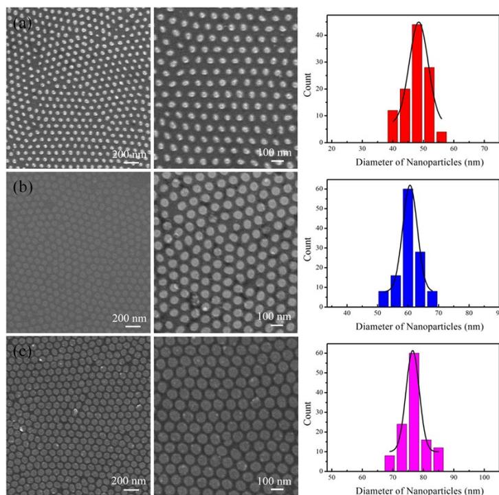
Fig. S1 SEM images of Ni NP arrays with three evaporation thickness of 10 nm (a), 15 nm (b) and 25 nm (c) and the according size distribution of diameter of the three Ni NP arrays.
