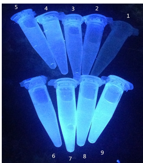
Figure S2. The photograph of the as-prepared products from different molar ratios of ammonia to CA with an irradiation of 365 nm UV light. The products were prepared by hydrothermal reaction of different molar ratios of ammonia to CA at 200 \text{ }^\circ\text{C} for 10 h. The molar ratios of ammonia to CA for 1 to 9 in the photograph are 0:1, 1:1.5, 1:3, 1:5, 1:8, 1.2:1, 3:1, 6:1, and 12:1, respectively.
