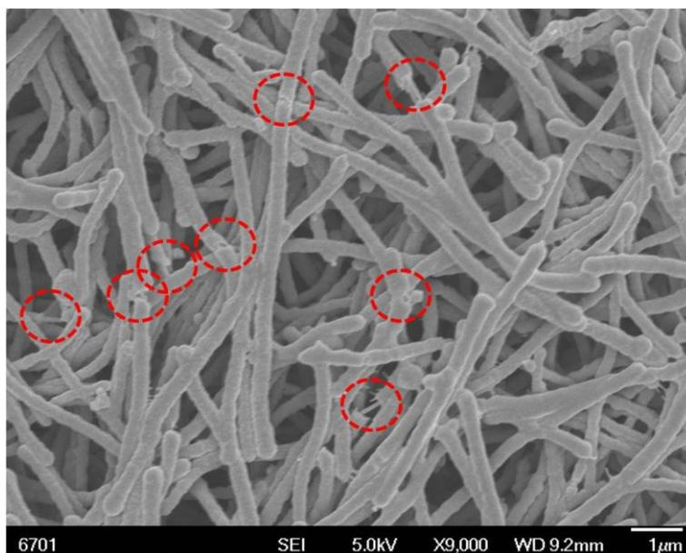
**Figure S2.** SEM image of Ag@TiO<sub>2</sub> core-shell nanowires prepared by hydrolysis reaction.
