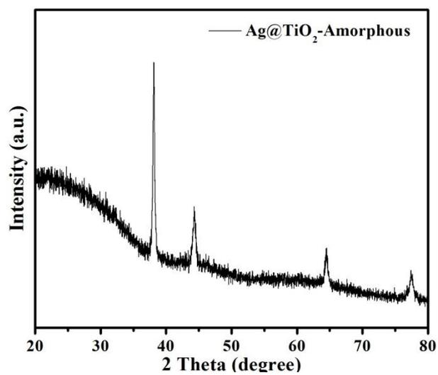
**Figure S3.** XRD patterns of the Ag@TiO<sub>2</sub>-amorphous core-shell nanowires.
