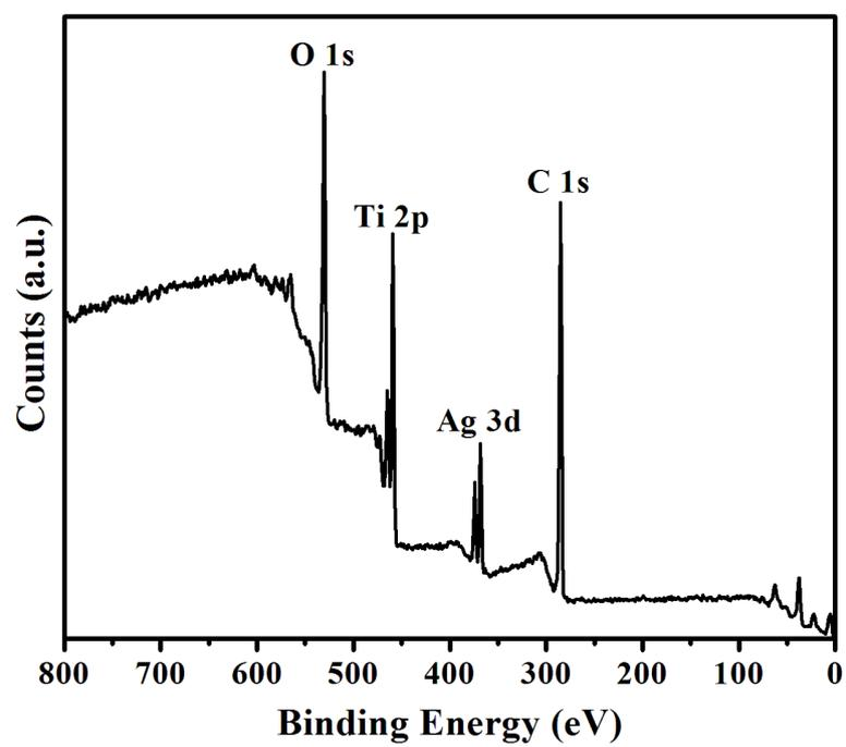
**Figure S1.** XPS spectra of the as-synthesized Ag@TiO<sub>2</sub> core-shell nanowires as shown in Figure 1B-D.
