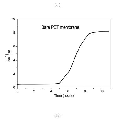
**Figure S1**: (a) Fluorescent intensities in the basolateral compartment of our microfluidic chip:  $I_{340}$  is increasing with time and  $I_{380}$  shows the opposite trend; (b) is the calculated ratio  $I_{340}/I_{380}$ .
