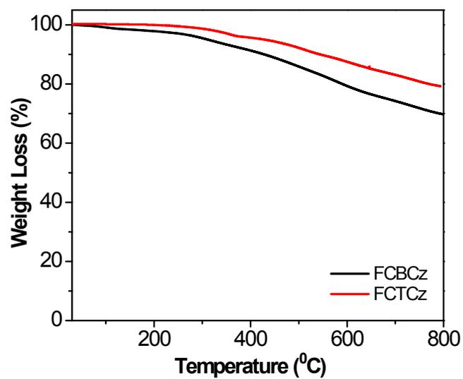
**Fig. S2.** Thermogravimetric analysis trace of the polymer networks under a nitrogen atmosphere with a heating rate of 10 °C/min.
