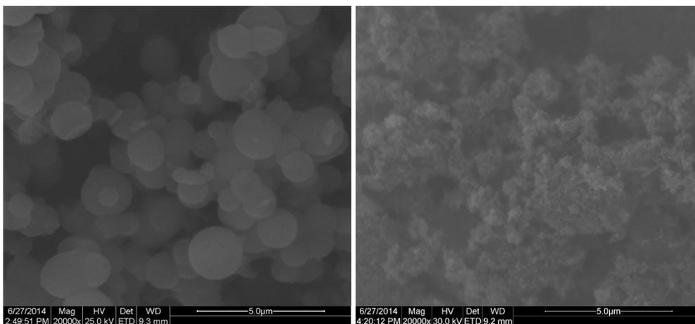
**Fig. S4.** Scanning electron microscopy (SEM) images for FCBCz (left) and FCTCz (right) with a scale bar of 5.0  $\mu\text{m}$ .
