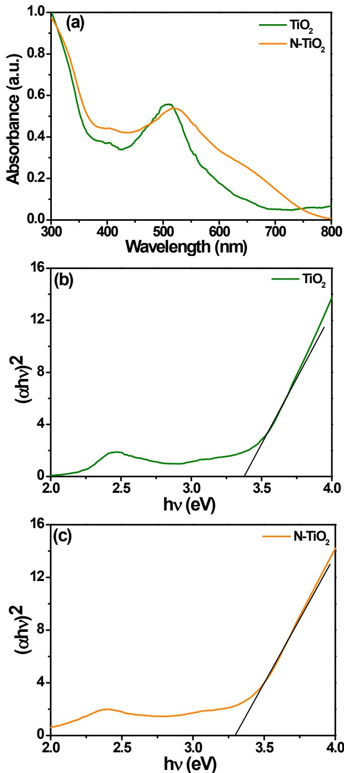
**Fig. S3 (a)** UV-visible absorption spectra of N719 dye adsorbed TiO<sub>2</sub> and N-TiO<sub>2</sub> photoanodes. Plots of  $(\alpha h\nu)^2$  vs.  $h\nu$  obtained for the N719 dye adsorbed (b) TiO<sub>2</sub> and (c) N-TiO<sub>2</sub> photoanodes.
