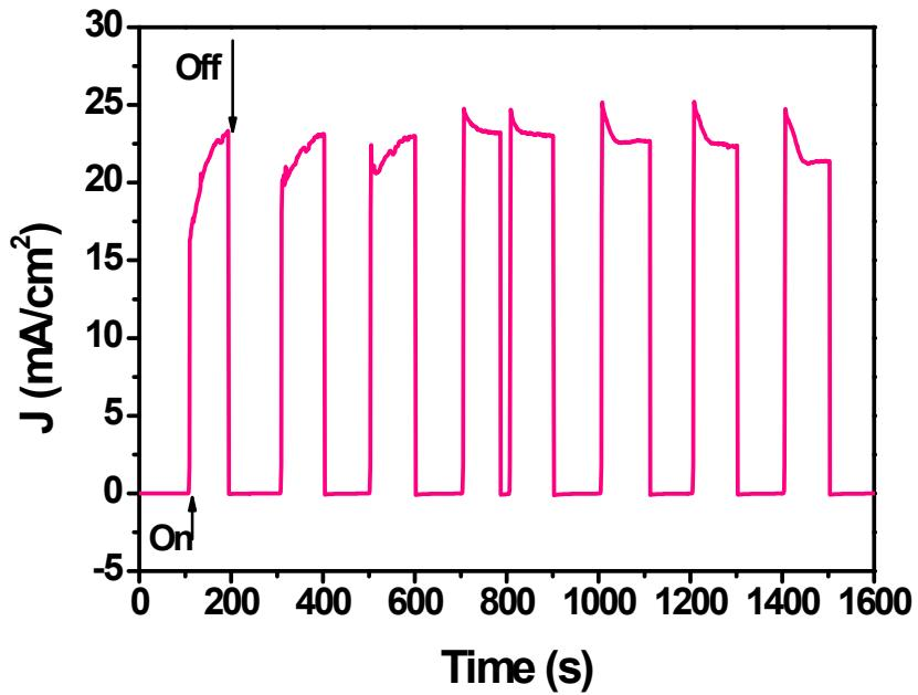
**Fig. S5.** Photocurrent density–time (J–T) profile obtained for the N-TiO<sub>2</sub>-Ag (10 wt.% of Ag) plasmonic photoanode modified DSSC under illumination ‘on-off’ condition.
