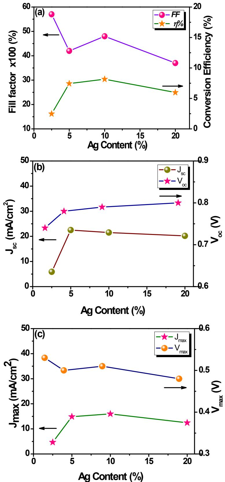
**Fig. S4.** Plots of **(a)** fill factor (FF) and power conversion efficiency ( $\eta$ ), **(b)** short-circuit current density ( $J_{sc}$ ) and open-circuit voltage ( $V_{oc}$ ), and **(c)** maximum photocurrent density ( $J_{max}$ ) and maximum photovoltage ( $V_{max}$ ) obtained for N-TiO<sub>2</sub>-Ag-based DSSC with different Ag contents.
