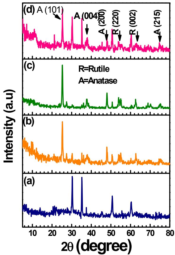
**Fig. S1.** X-ray diffraction patterns of (a) ITO, (b)  $\text{TiO}_2$ , (c) N- $\text{TiO}_2$ , and (d) N- $\text{TiO}_2$ -Ag.
