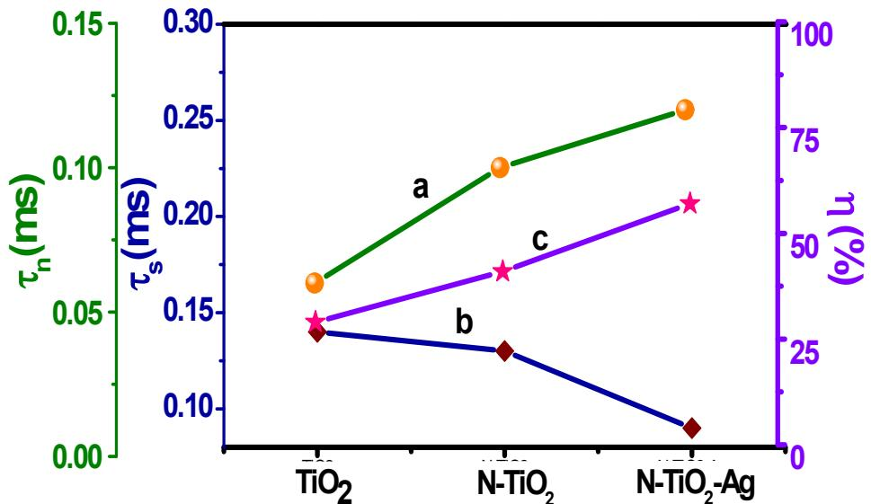
**Fig. S6.** (a) Electron lifetime ( $\tau_n$ ), (b) electron transport time ( $\tau_s$ ), and (c) charge collection efficiency ( $\eta_c$ ) of TiO<sub>2</sub>, N-TiO<sub>2</sub>, and N-TiO<sub>2</sub>-Ag photoanode-based DSSCs.
