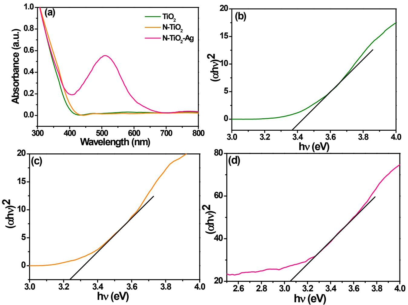
**Fig. S2** (a) UV-visible absorption spectra of  $\text{TiO}_2$ , N- $\text{TiO}_2$ , and N- $\text{TiO}_2$ -Ag. Plots of  $(\alpha h\nu)^2$  versus  $h\nu$  obtained for (b)  $\text{TiO}_2$ , (c) N- $\text{TiO}_2$ , and (d) N- $\text{TiO}_2$ -Ag.
