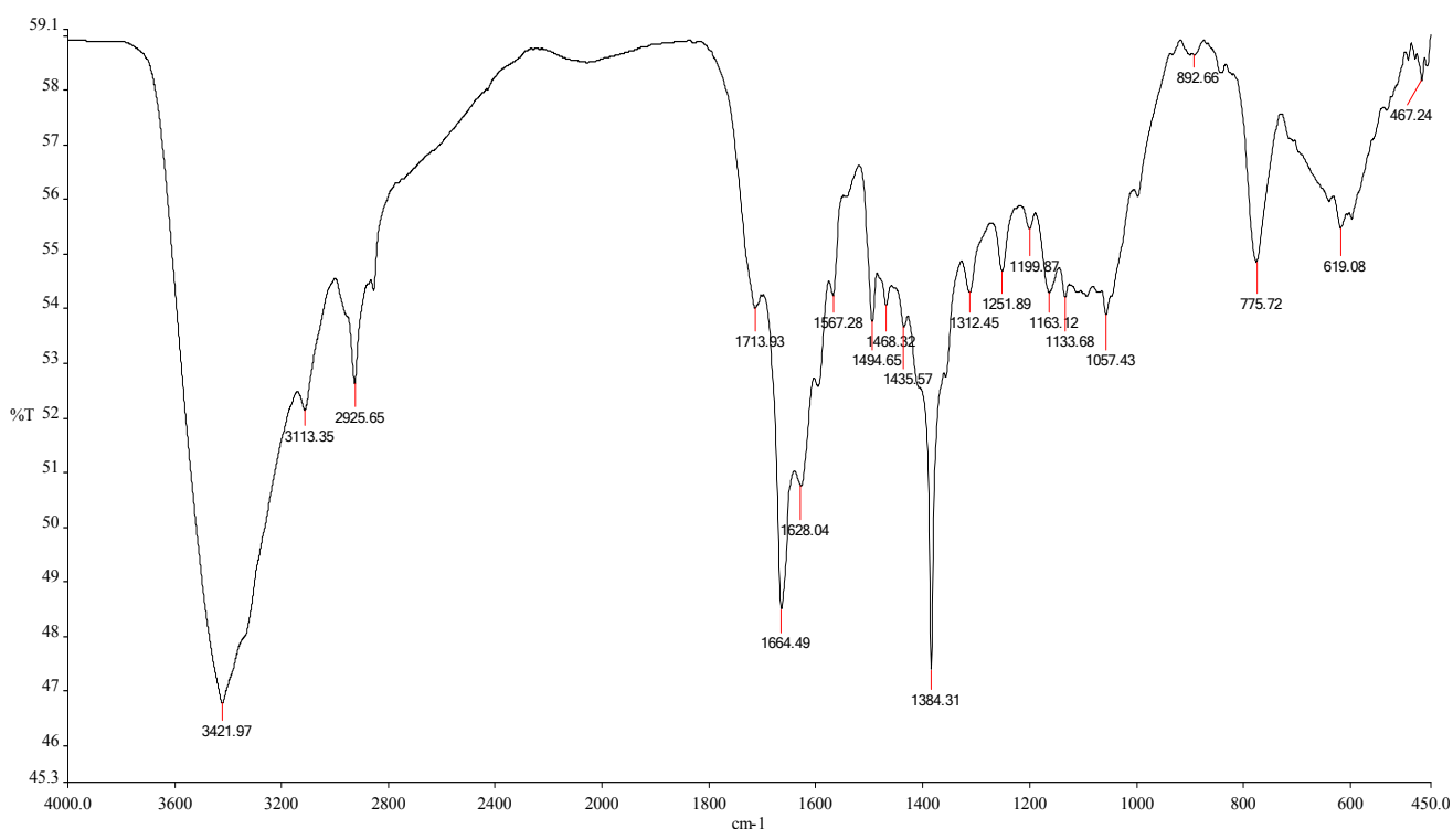
Fig. S1 FTIR spectrum of the ligand H 3 phpda in the region of 4000-450 cm -1 .
