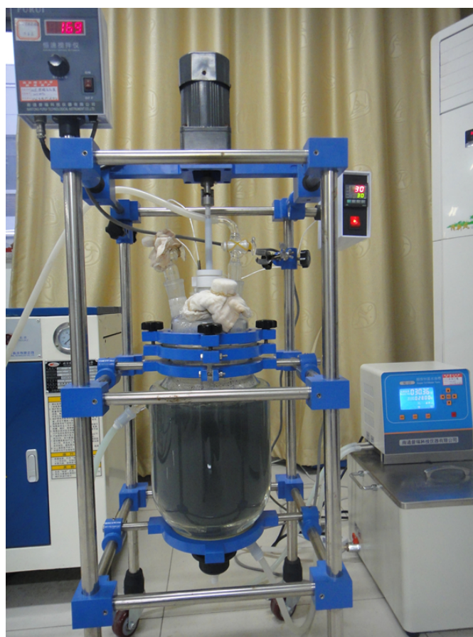
Figure S-2. Bio-oxidation of graphite by Acidithiobacillus ferrooxidans CFMI-1 using a 5 L glass reaction kettle.
