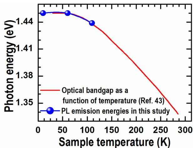
Figure S6: Comparisons of the measured PL emission energies in this study with those of optical bandgap energies reproduced with permission from Ref. 43.
