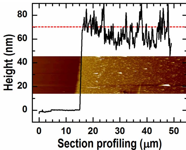
Figure S5: Thickness measurement of the sulfurized Bi<sub>2</sub>S<sub>3</sub> thin film by AFM from the edge of an intentionally starched area.
