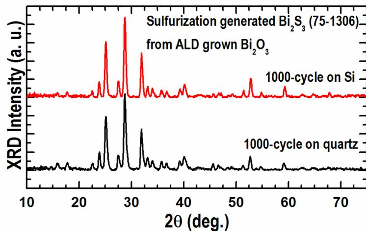
Figure S4: XRD patterns collected from the sulfurized (at 500 °C) Bi<sub>2</sub>S<sub>3</sub> thin films with the initial Bi<sub>2</sub>O<sub>3</sub> grown by ALD on Si and quartz substrates.
