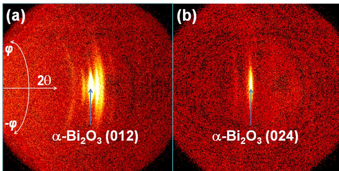
Figure S1: XRD area imaging of the diffraction intensity distributions in  $\varphi$ - $2\theta$  frames (a) targeting the  $\alpha\text{-Bi}_2\text{O}_3$  (012) diffractions and (b) targeting at the  $\alpha\text{-Bi}_2\text{O}_3$  (024) diffractions.
