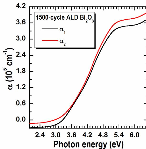
Figure S7: Absorption coefficient spectra of 1500-cycle ALD grown  $\text{Bi}_2\text{O}_3$  obtained
