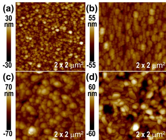
Figure S3: AFM images recorded from the sulfurized Bi<sub>2</sub>O<sub>3</sub> samples, i.e., the Bi<sub>2</sub>O<sub>3</sub> thin film samples after sulfurization, on quartz substrates: (a) 500 cycles sulfurized at 500 °C, (b) 1000 cycles sulfurized at 500 °C, (c) 1500 cycles sulfurized at 500 °C, and (d) 1500 cycles sulfurized at 600 °C.
