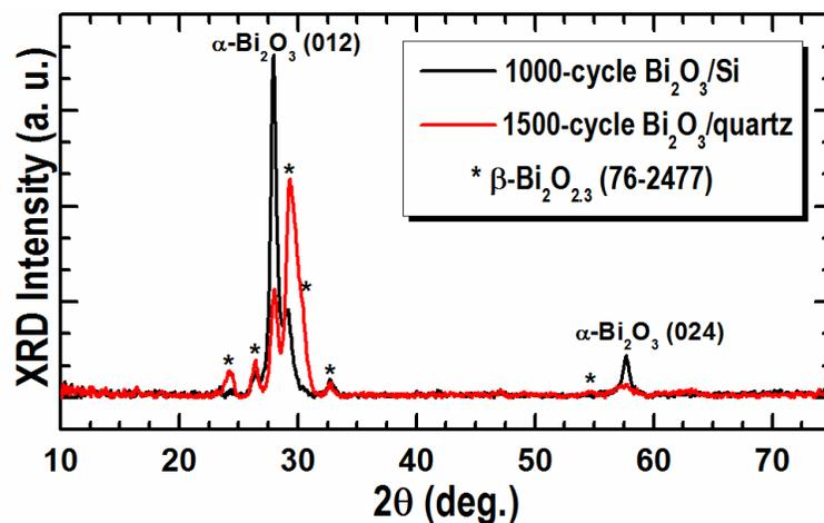
Figure S2: XRD patterns collected from the Bi<sub>2</sub>O<sub>3</sub> thin film samples grown by ALD on Si and quartz substrates.
