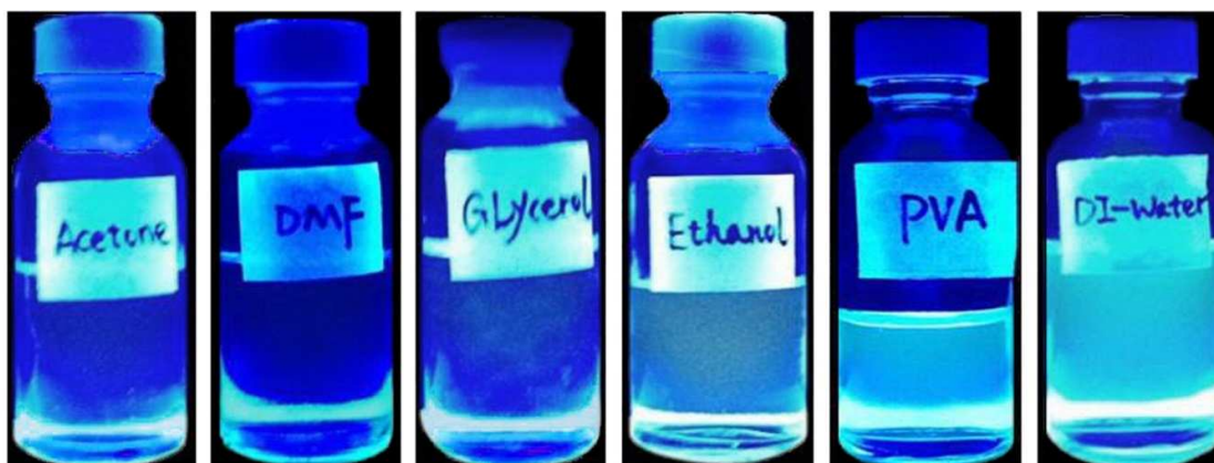
Figure S7 The solubility and PL of obtained GQDs in different solvents, and the solvents are acetone, DMF, glycerol, ethanol, PVA and DI-water in turn
