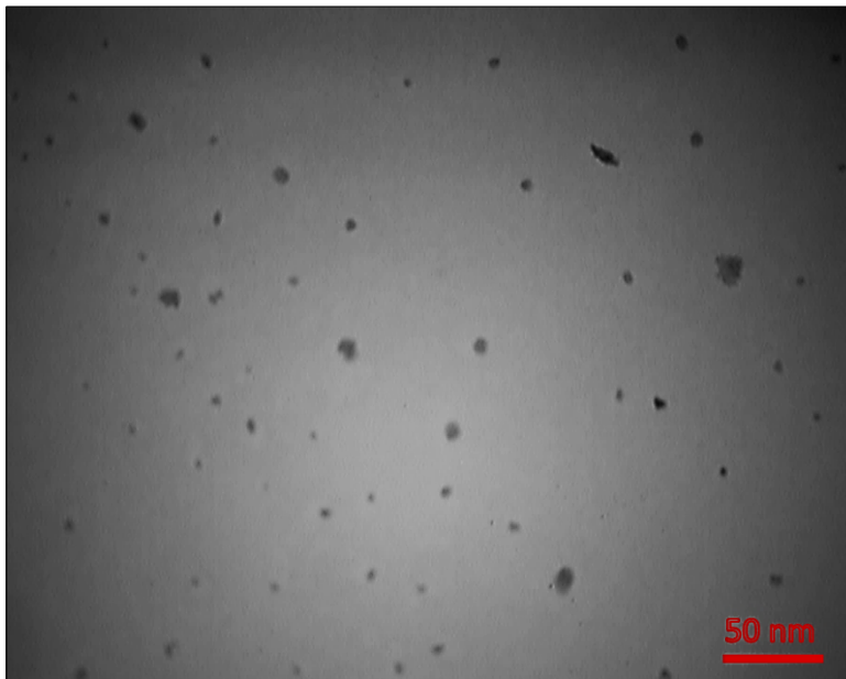
Figure S2. TEM image of titania nanoparticles formed in micelle nanoreactors, scale bar 50 nm.
