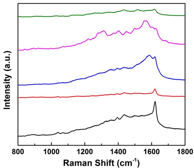
**Fig. S5** SERS spectra of methylene blue (MB,  $10^{-6}$  mol/L) taken from different sites on the Ag nanoparticle assemblies supported on  $\text{Cu}_2\text{O}$  crystals prepared using lactic acid as the additive acid.
