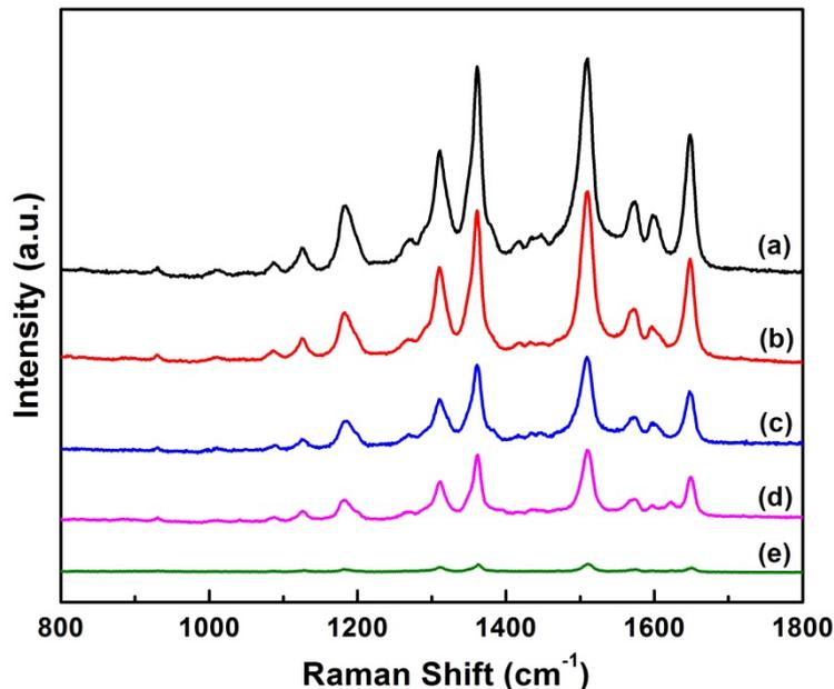
**Fig. S4** SERS spectra of RhB of different concentrations measured on Ag nanoparticle assemblies obtained from galvanic replacement for 30 s: (a)  $10^{-5}$ , (b)  $10^{-6}$ , (c)  $10^{-7}$ , (d)  $10^{-8}$ , (e)  $10^{-9}$  mol/L.
