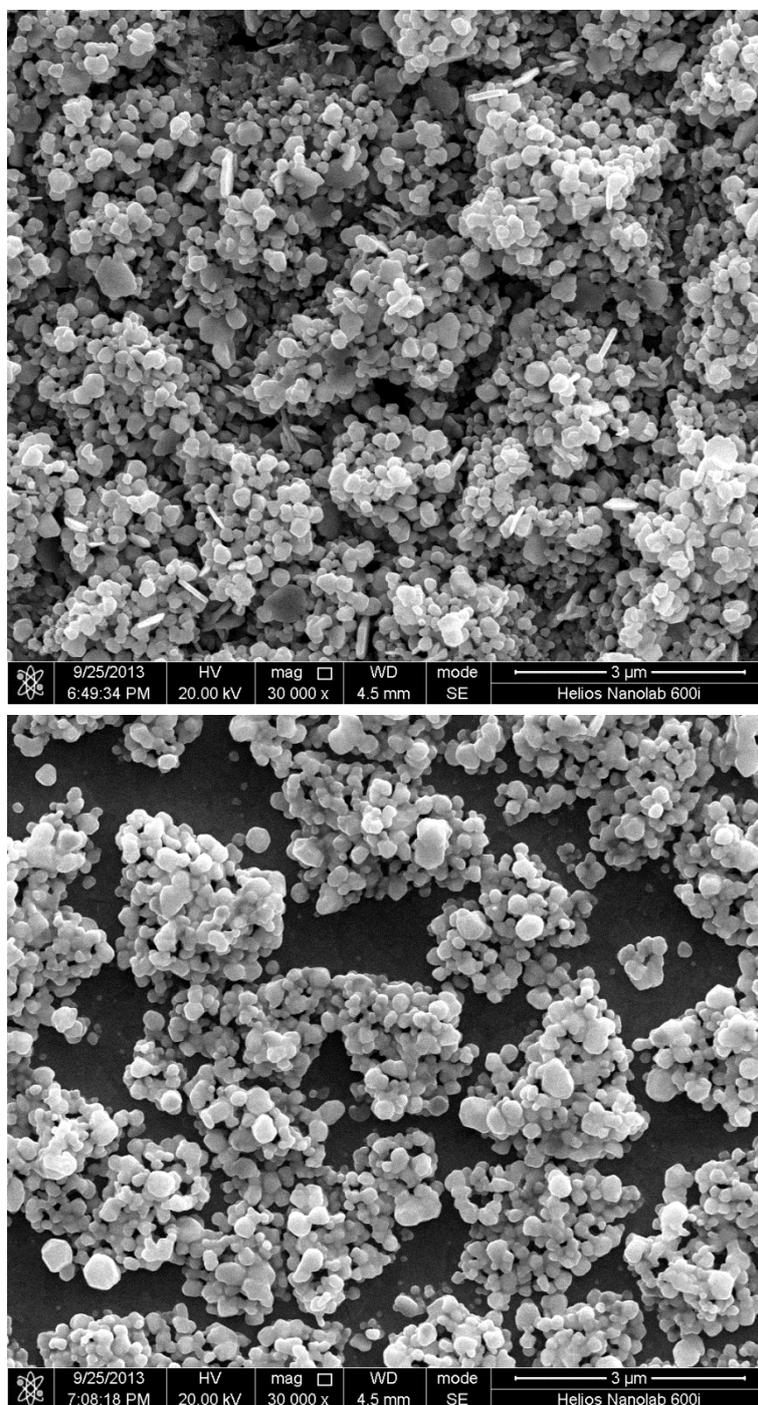
**Fig. S1** SEM images of Ag nanoparticle assemblies obtained from galvanic replacement for (top) 5 min, and (down) 10 min. During the galvanic replacement process, 5-sulfosalicylic acid was used as the additive acid.
