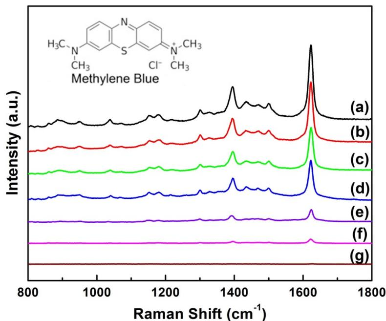
**Fig. S3** SERS spectra of methylene blue (MB) of different concentrations measured on Ag nanoparticle assemblies obtained from galvanic replacement for 30 s (see Fig. 1e, f): (a)  $10^{-4}$ , (b)  $10^{-5}$ , (c)  $10^{-6}$ , (d)  $10^{-7}$ , (e)  $10^{-8}$ , (f)  $10^{-9}$ , (g)  $10^{-10}$  mol/L.
