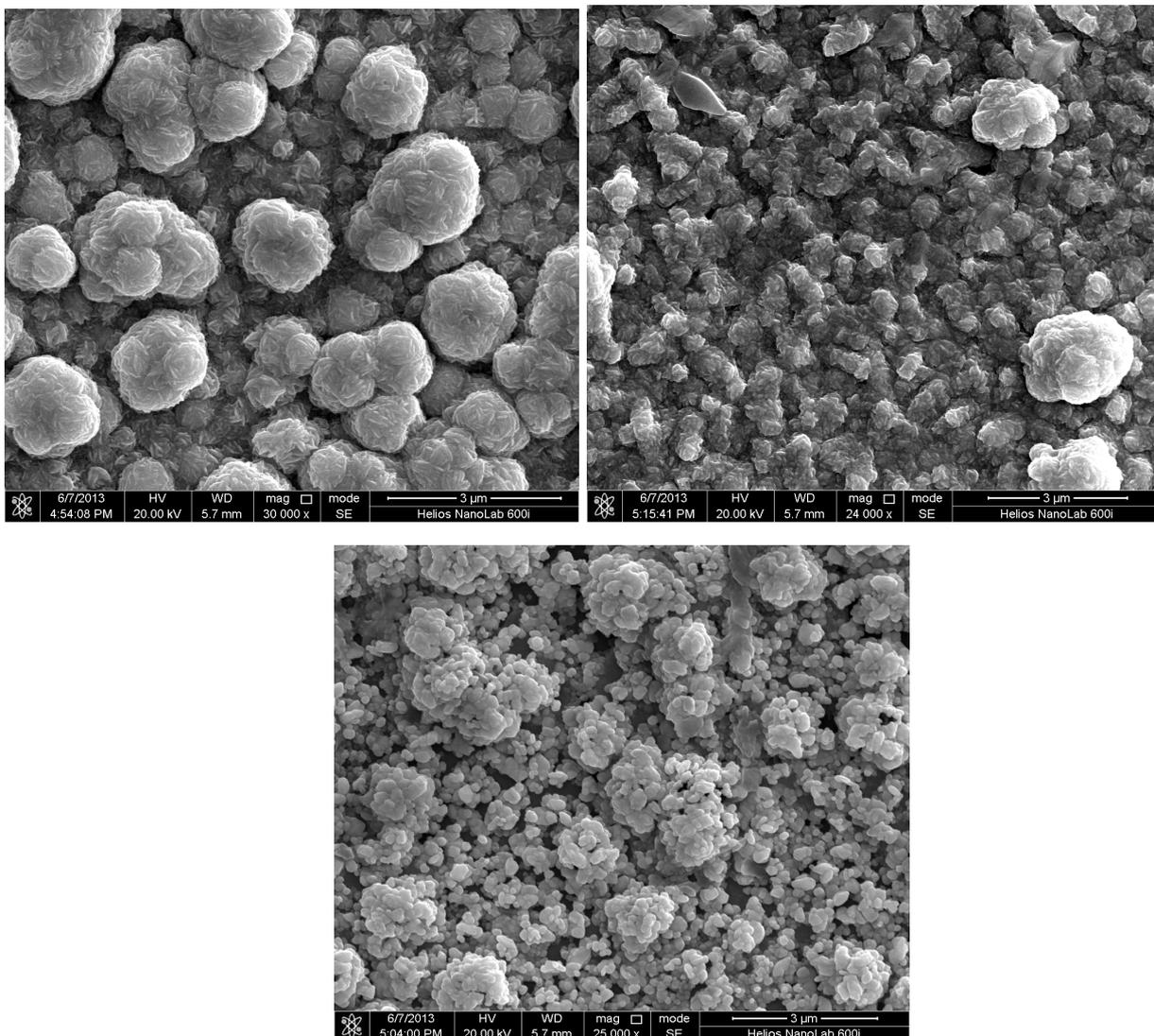
**Fig. S2** SEM images of Ag nanoparticle assemblies obtained from galvanic replacement for 30 s. During the galvanic replacement process, citric acid (up, left), camphorsulfonic acid (up, right), and lactic acid (down) were used as the additive acid.
