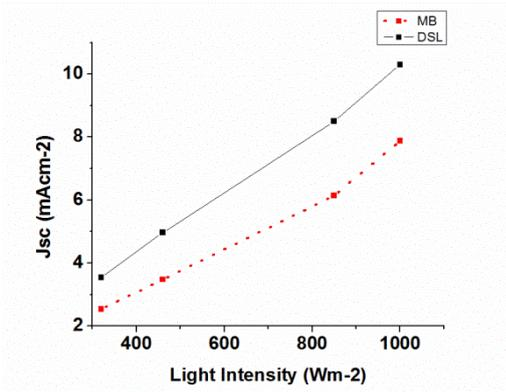
**Fig. S4.**  $J_{sc}$  versus light intensity for fabricated devices.
