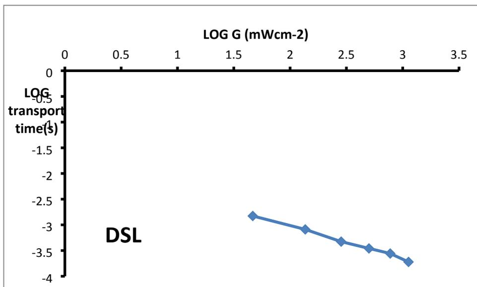
**Fig. S7.** Log-Log plots of transport time versus light intensity for MB and DSL cells.
