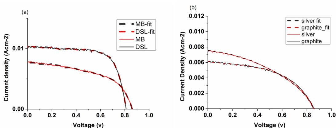
**Fig. S8.** Measured and fitted I-V curve for the a) MB and DSL device presented in main article. b) silver and graphite devices presented in supporting information.
