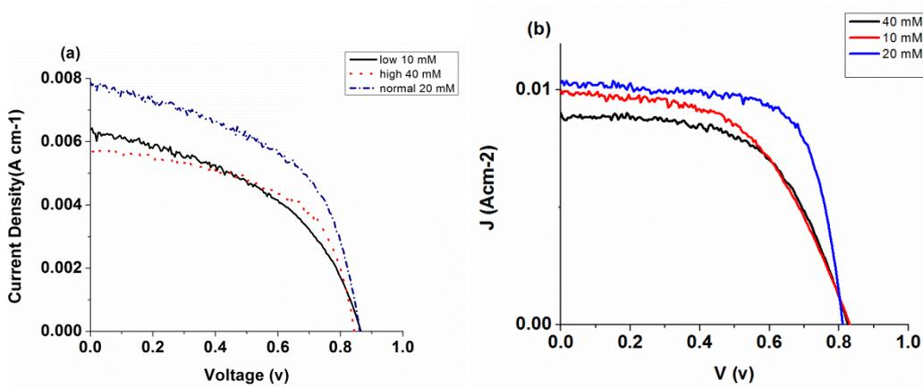
**Fig. S5-** IV curves of the devices with different Li concentrations for a) MB and b) DSL devices.
