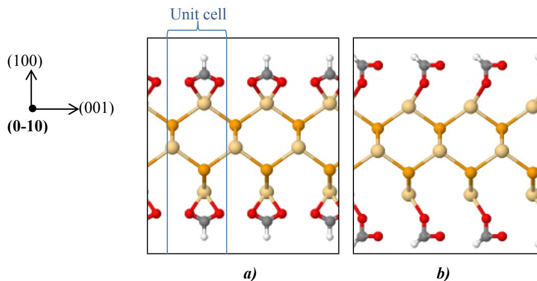
**Figure S2.** Initial geometries of CdSe.HCOO with a) bidentate and b) monodentate adsorption mode of the HCOO<sup>-</sup> ligand.
