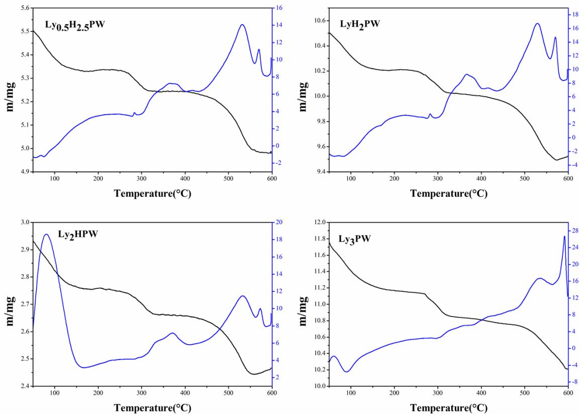
**Fig. S4** The thermal analysis (TG/DTA) curves of  $\text{Ly}_{3-x}\text{H}_x\text{PW}$ .
