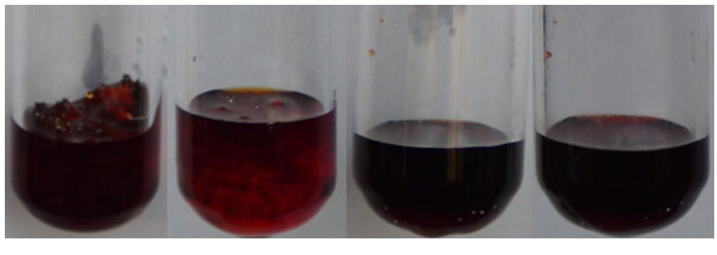
**Fig. S5** The different fructose/ChCl weight ratio of fructose conversion. Reaction conditions: 110 °C in 1 min. a. fructose/ChCl weight ratio is 2:6; b. fructose/ChCl weight ratio is 3:6; c. fructose/ChCl weight ratio is 4:6; d. fructose/ChCl weight ratio is 5:6.
