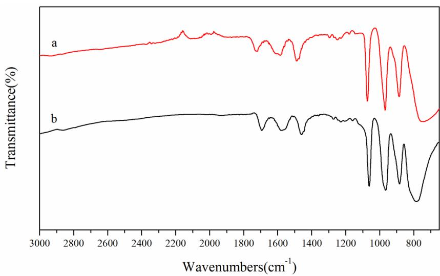
**Fig. S6** The IR spectra of Ly<sub>2</sub>HPW (a) and reused Ly<sub>2</sub>HPW (b).
