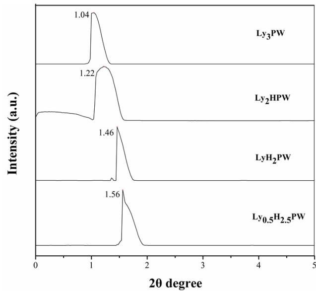
**Fig. S3** Low-angle XRD patterns of  $\text{Ly}_{3-x}\text{H}_x\text{PW}$ .
