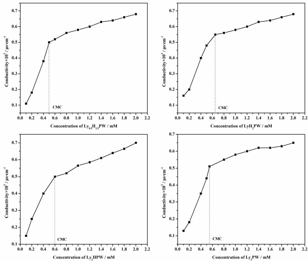
**Fig. S2** The CMC of  $\text{Ly}_{3-x}\text{H}_x\text{PW}$  in room temperature
