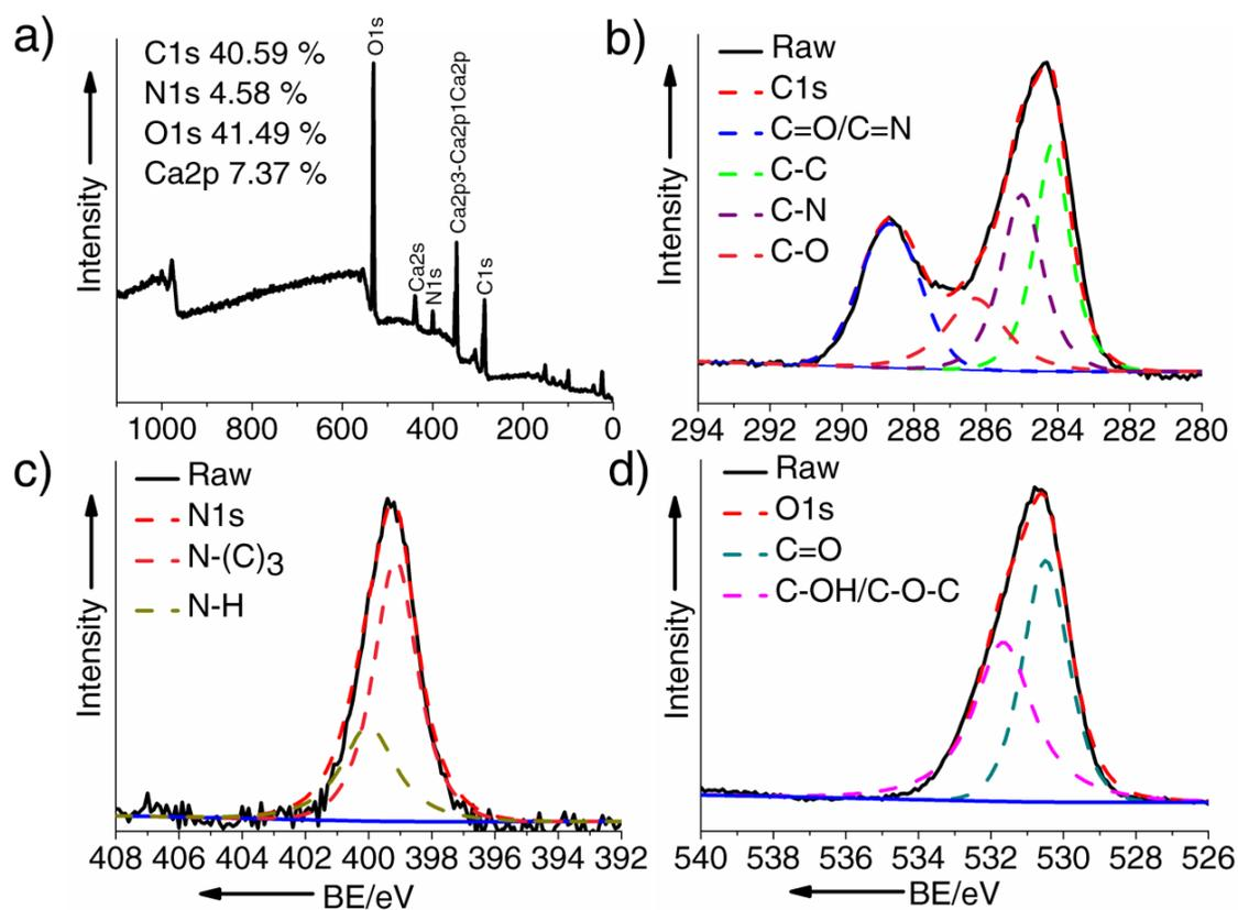
**Fig. S5.** XPS spectra of the eggshell powder. (a) Survey spectrum. (b)-(d) High resolution spectrum of (b) C1s, (c) N1s, and (d) O1s.
