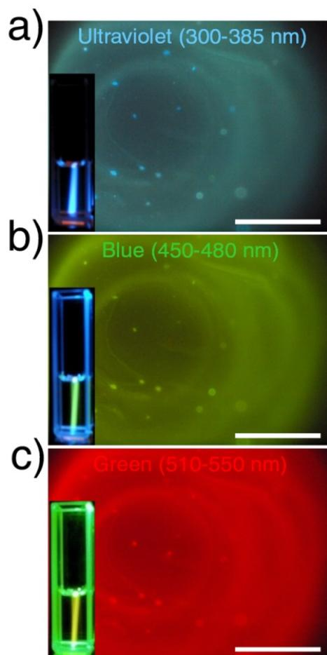
**Fig. S8.** Multicolor fluorescence images of **NCND 2** on glass plate under excitation at UV (300-385 nm), blue (450-480 nm), and green (510-550 nm) light; inset shows the corresponding fluorescence images of **NCND 2** in aqueous solution.
