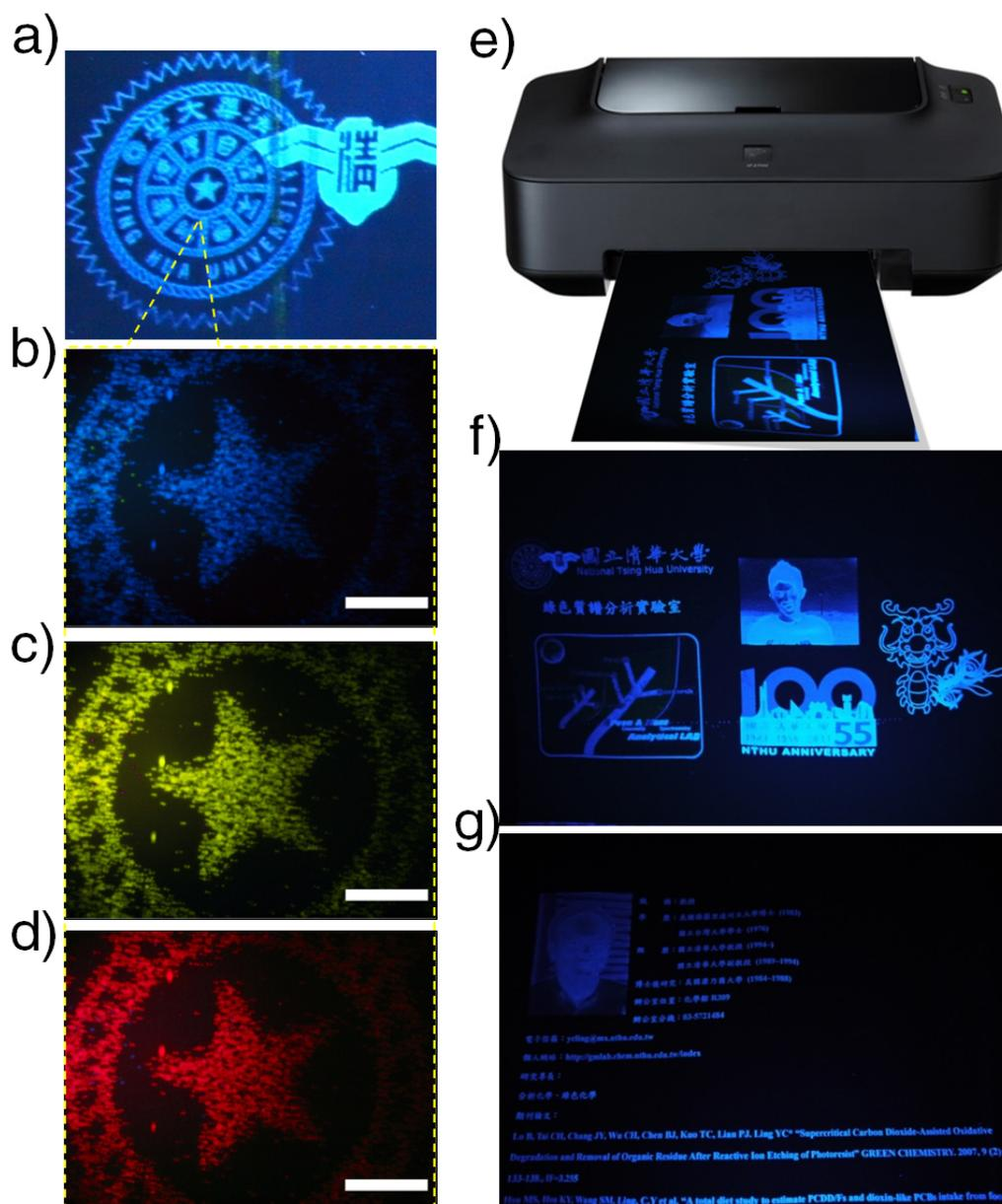
**Fig. S15.** Different graphic patterns (a, e, and f) and resume (g) obtained by **NCND 2** ink under the UV light excitation. Fluorescent images (b-d) captured under UV (300-385 nm), blue (450-480 nm) and green (510-550 nm) light excitation.
