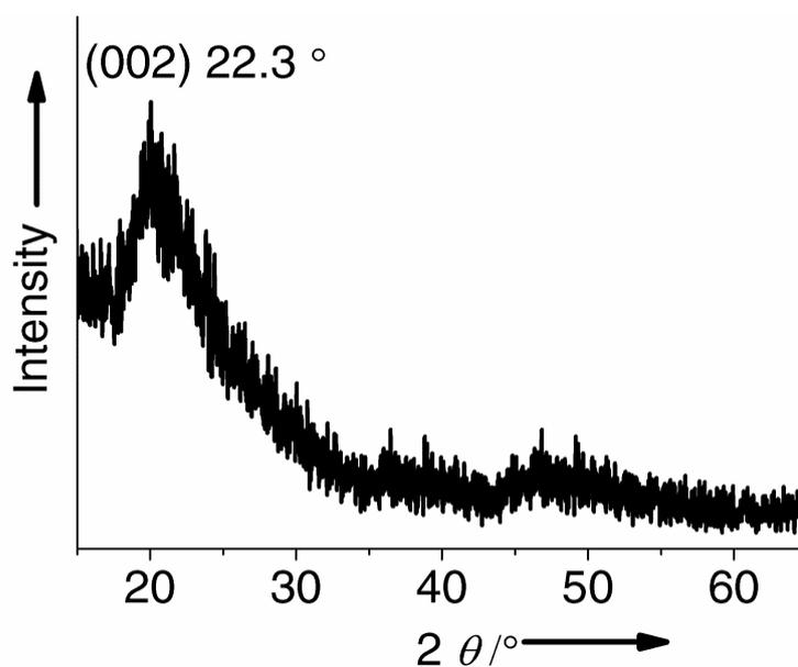
**Fig. S1.** The XRD spectrum of NCND 2.
