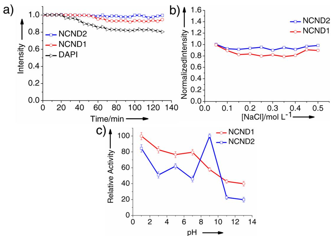
**Fig. S9.** The photostabilities of **NCND 1** and **NCND 2**. (a) Effects of irradiation time on the fluorescence intensity of **NCND 1** (red), **NCND 2** (blue), and an organic fluorophore, DAPI (black). (b) Effect of ionic strengths on the fluorescence intensity of **NCND 1** (red) and **NCND 2** (blue); the ionic strength were controlled by various concentrations of NaCl. (c) Effect of pH on the fluorescence intensity of **NCND 1** (red) and **NCND 2** (blue).
