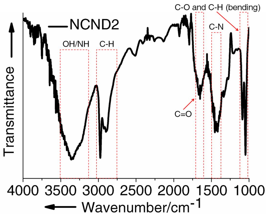
Fig. S3. The FTIR spectrum of NCND 2.
