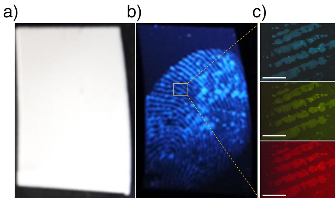
**Fig. S16.** An NCND 2 formed fluorescent fingerprint on commercially available filter paper captured under (a) daylight (b) UV light ( $\lambda_{\text{ex}} = 350$  nm) and (c) UV (300-385 nm), blue (450-480 nm), and green (510-550 nm) light excitation, respectively.
