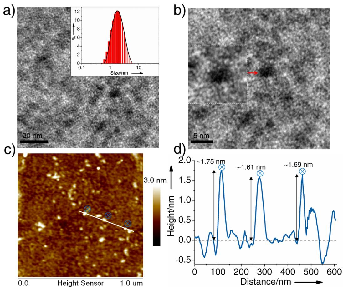
**Fig. S2.** (a) TEM image of as-prepared **NCND 1**; scale bar 20 nm (inset: the corresponding size distribution histograms). (b) HRTEM image of **NCND 1**; scale bar 5 nm. (c) AFM image of **NCND 1** on a silicon substrate. (d) The corresponding height-profile analysis along the line in (c).
