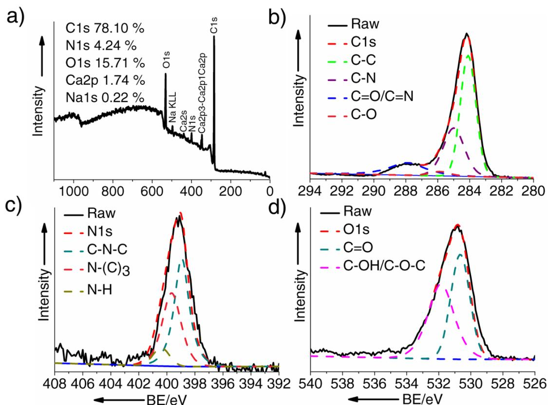
**Fig. S6.** XPS spectra of **NCND 1**. (a) Survey spectrum. (b)-(d) High resolution spectrum of (b) C1s, (c) N1s, and (d) O1s.
