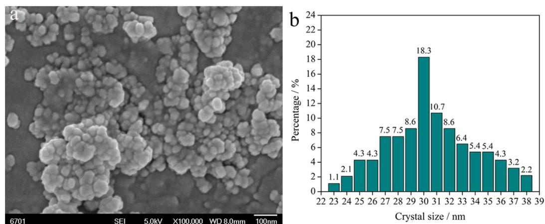
**Fig. S1** (a) SEM image of the nano SiO<sub>2</sub>, scale bar: 100 nm. (b) Particle size distribution of nano SiO<sub>2</sub> analysed from SEM image.
