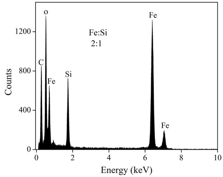
**Fig. S2** EDX spectrum of Fayalite@C nanocomposites, in which the Cu signal originated from the Cu grid support for TEM observation.
