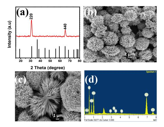
Fig. 1: (a) XRD pattern of ZnCO<sub>2</sub>O<sub>4</sub> grown on ITO coated with ZnO seed layer showing preferential growth along 220. Low (b) and high (c) magnification FESEM images of the sample. (d) EDS spectra showing composition of the sample and traces of substrate.
