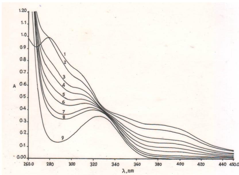
5 Figure S2- Successive Spectral Scans for Reduction of *trans*-Mn<sup>III</sup>(salen)(OH<sub>2</sub>)<sub>2</sub><sup>+</sup> by Oxalate.
