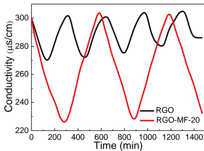
**Fig. S9** The regeneration cycles of the RGO and RGO-MF-20 electrodes with the absence of an external potential.
