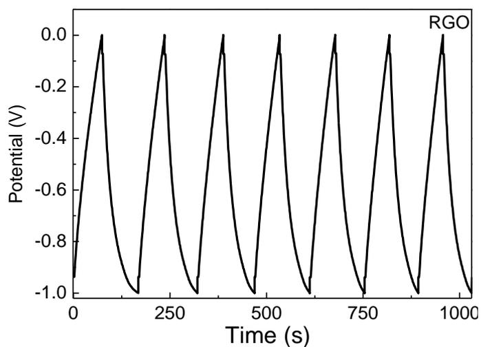
**Fig. S8** Continuous GC curves of the RGO electrode with a current density of 0.3 A/g.
