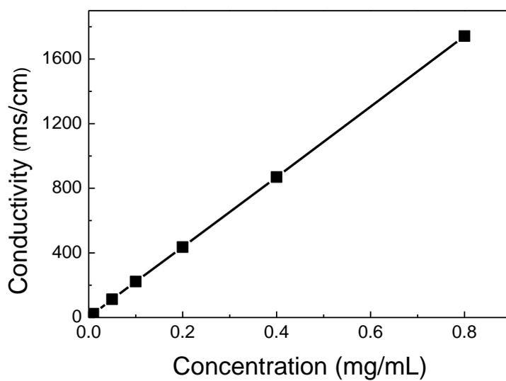
**Fig. S2** The relationship between conductivity and concentration of NaCl solutions.
