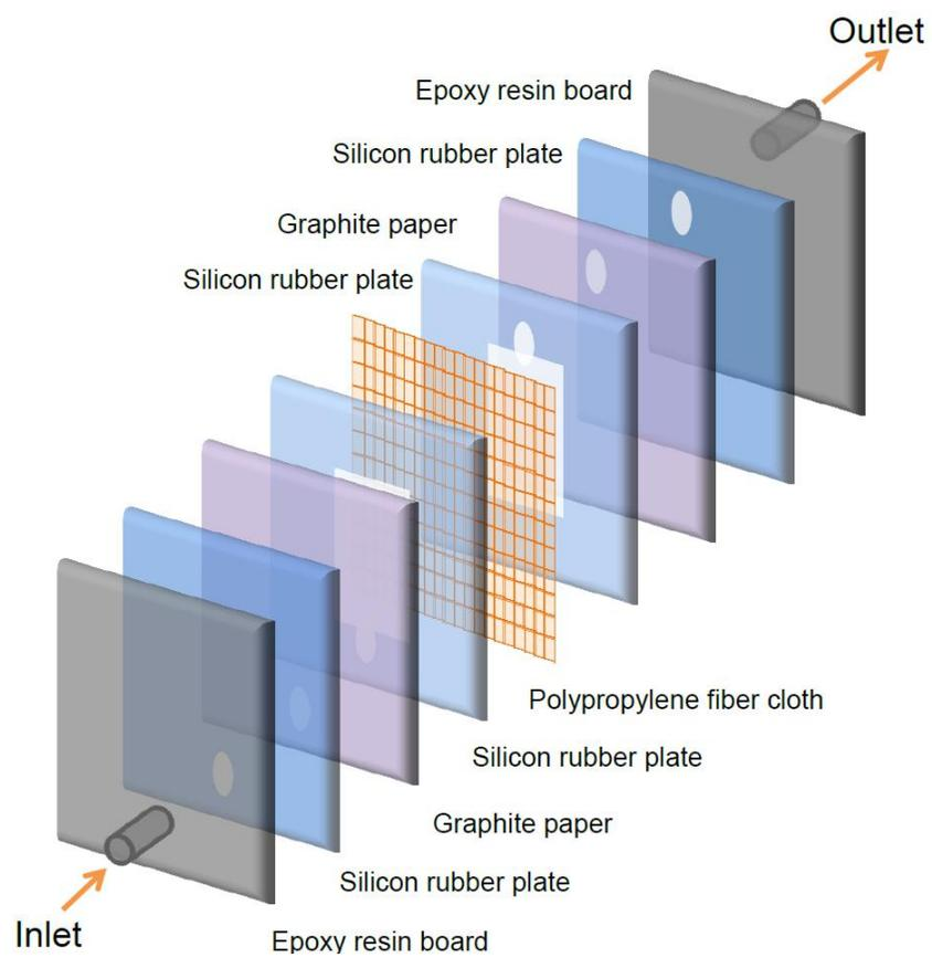
**Scheme S1.** Schematic illustration of CDI device.
