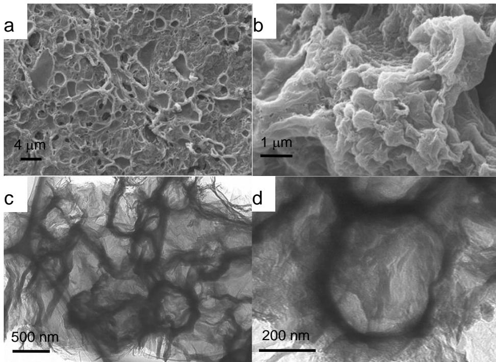
**Fig. S4** (a,b) SEM and (c,d) TEM images of 3D RGO-MF-20 composite.
