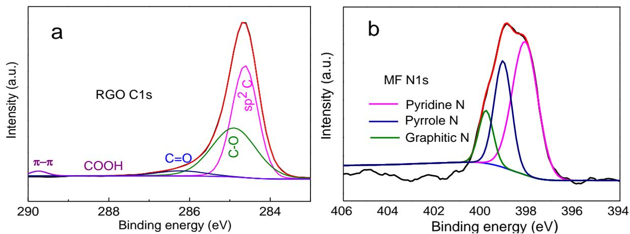
Fig. S6 (a) XPS C1s core level spectra of RGO and (b) XPS N1s core level spectra of MF.
