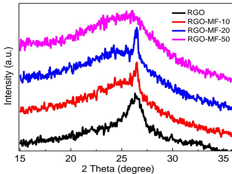
Fig. S5 XRD patterns of RGO and RGO-MF composites.
