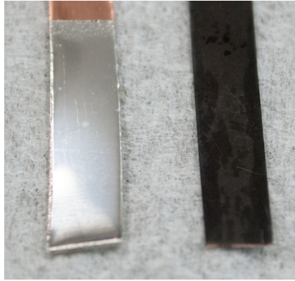
Fig. S1 Photograph of electrodeposited Ni (left) and electroless deposited Ni (right).
