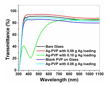
Wavelength vs. transmittance plots for bare glass, blank PVP on glass and PVP films with different Ag loadings deposited on glass.
