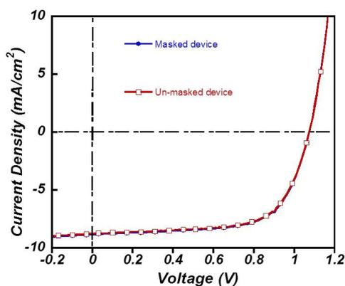
**Figure S4** Current density–Voltage ( $J$ - $V$ ) characteristics for planar heterojunction solar cells based on the masked and un-masked devices architecture.
