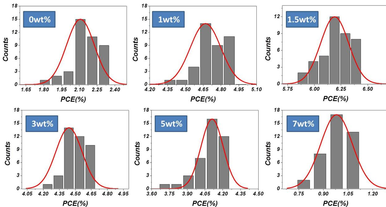
**Figure S6.** Histogram of solar cell efficiencies measured for 40 ITO/PEDOT:PSS/Perovskite-PEOXA/PCBM/Al devices with increasing the weight percent of PEOXA in GBL solvent.
