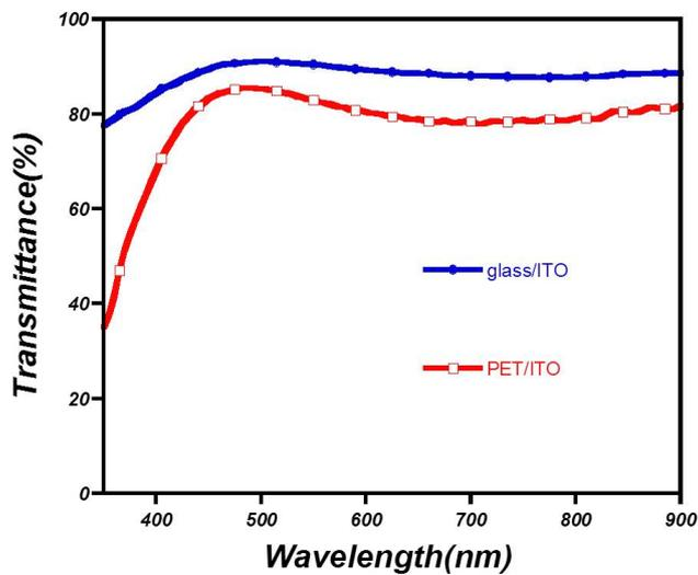
**Figure S7.** The optical transmittance of the Glass/ITO substrate together with the PET/ITO substrate
