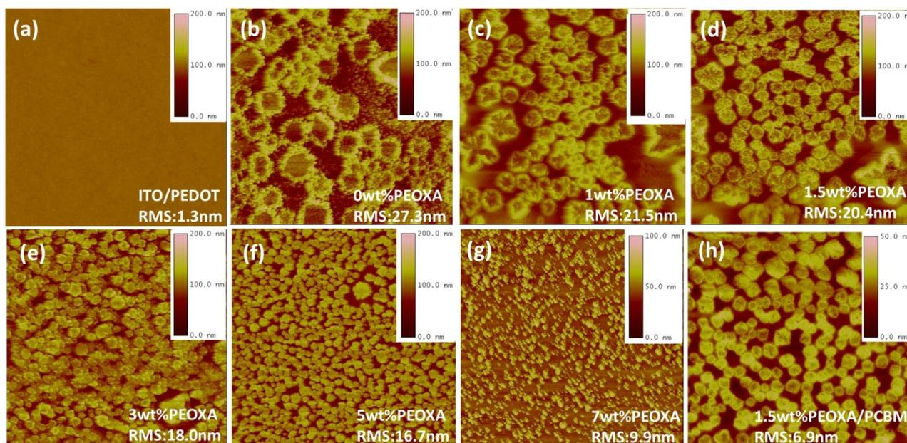
**Figure S1.** Topographic AFM images for  $\text{CH}_3\text{NH}_3\text{PbI}_3$ -PEOXA prepared from GBL solvent with increasing the weight percent of PEOXA and  $\text{CH}_3\text{NH}_3\text{PbI}_3$ -1.5wt% PEOXA /PC<sub>61</sub>BM film on the ITO/PEDOT:PSS substrate respectively. All the images are 20 $\mu\text{m}$ ×20 $\mu\text{m}$ .
