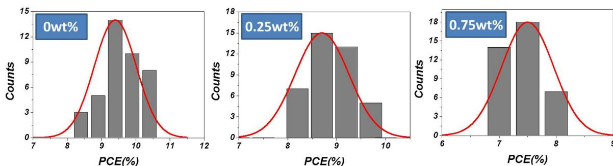
**Figure S3.** Histogram of solar cell efficiencies measured for 40 ITO/PEDOT:PSS/ $\text{CH}_3\text{NH}_3\text{PbI}_x\text{Cl}_{3-x}$ -PEOXA/PCBM/Al devices with increasing the weight percent of PEOXA in DMF solvent.
