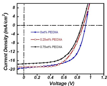
**Figure S2** Current density–Voltage (J-V) characteristics for  $\text{CH}_3\text{NH}_3\text{PbI}_x\text{Cl}_{3-x}$ -PEOXA composite film with increasing the weight percent of PEOXA in DMF solvent.
