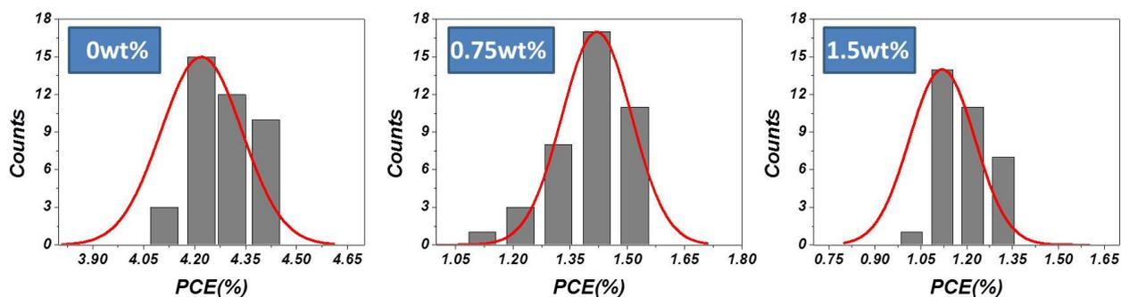
**Figure S5.** Histogram of solar cell efficiencies measured for 40 ITO/PEDOT:PSS/Perovskite-PEOXA/PCBM/Al devices with increasing the weight percent of PEOXA in DMF solvent.
