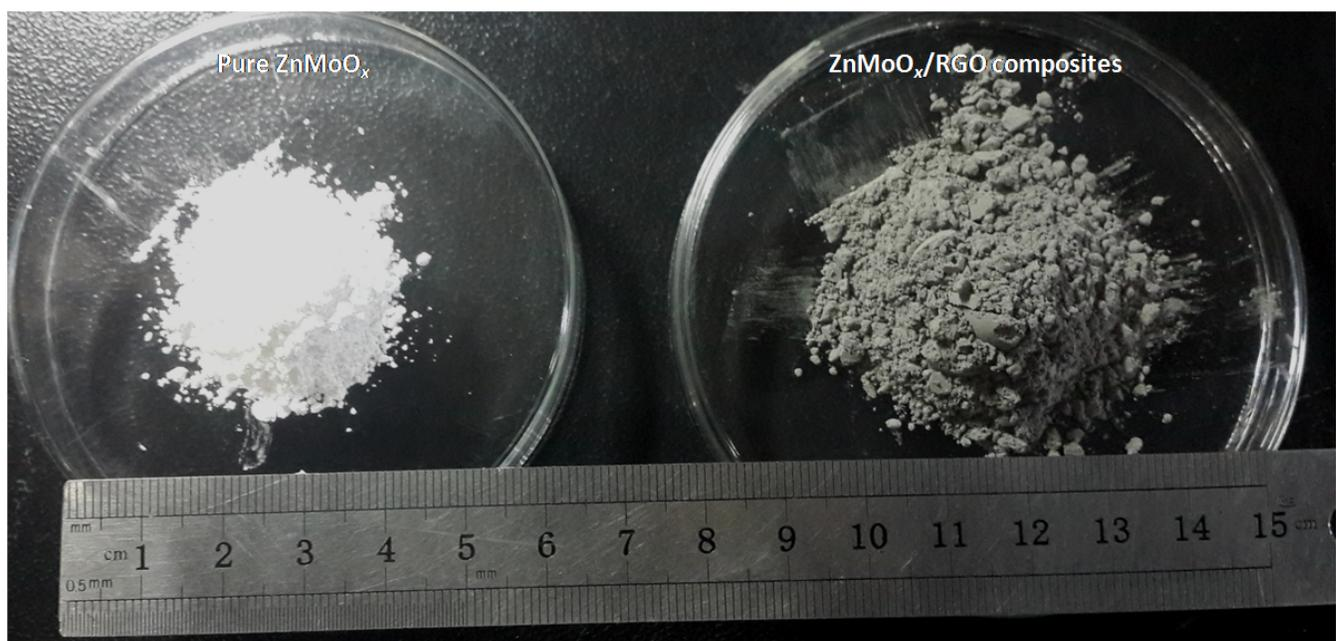
**Figure S1. Photograph showing the appearance of pure ZnMoO<sub>x</sub> (MG-0) and ZnMoO<sub>x</sub>/RGO composites (MG-3).**
