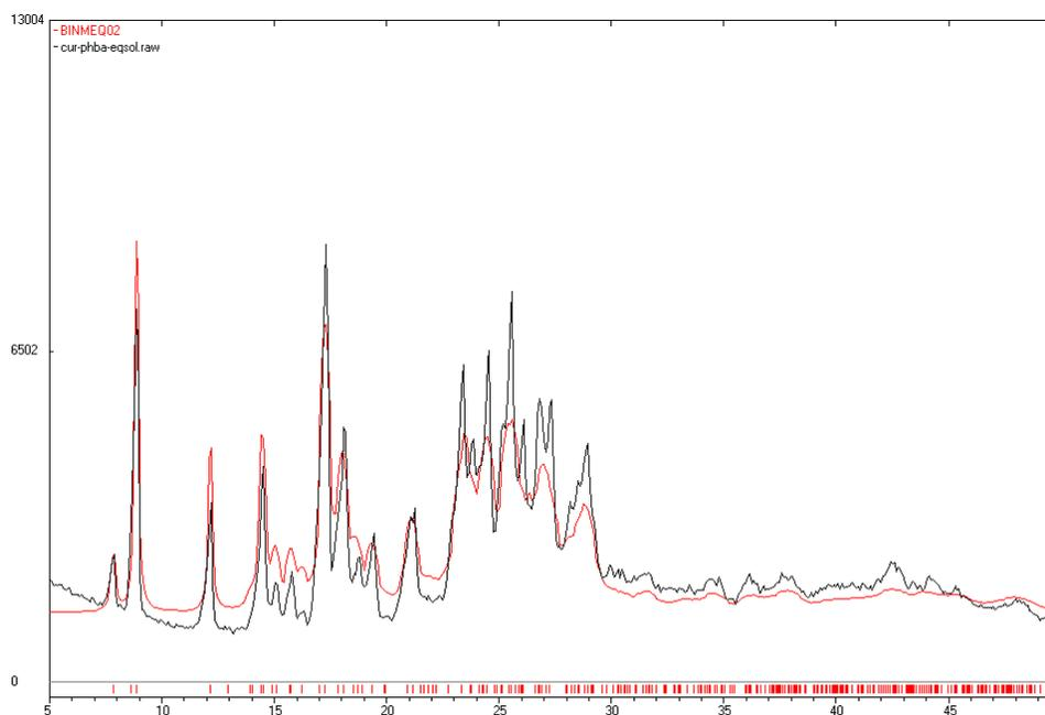
**Figure S9d** PXR D of CUR at the end of IDR experiment matches with calculated XRD lines of curcumin form I.
