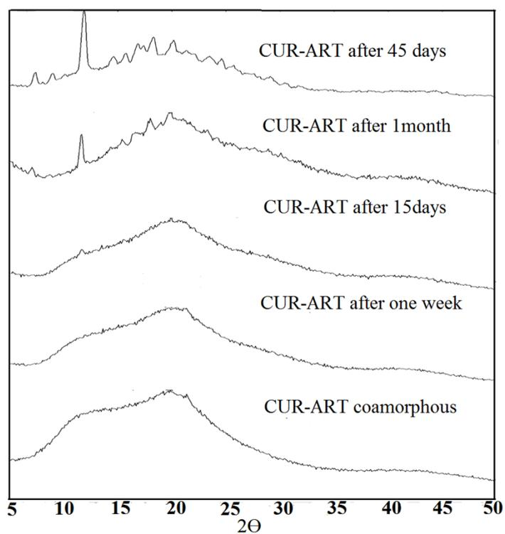
**Figure S8** PXRD plots CUR-ART kept in the stability chamber at  $40\text{ }^{\circ}\text{C}$  and 75% RH for 45 days.
