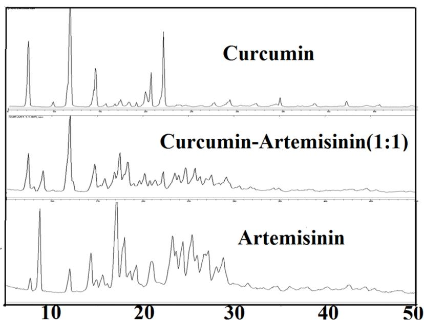
**Figure S9f** PXRD of CUR-ART coamorphous at the end of IDR experiment matches with starting materials like physical mixture of CUR-ART.
