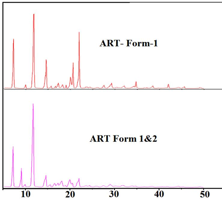
**Figure S5** PXR D pattern of ART Form 1 and mixture of ART Form 1 and 2 obtained by rotavaporization.
