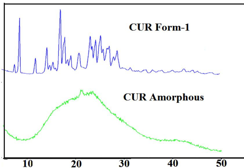
**Figure S4** PXRD pattern CUR crystalline and CUR amorphous forms obtained by rotavaporization.
