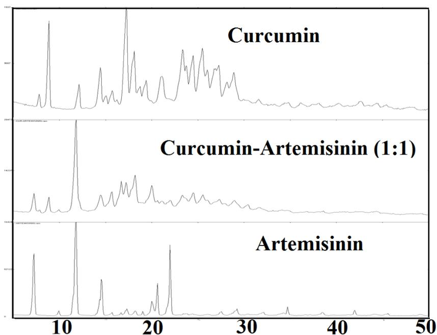
**Figure S1a** Curcumin-Artemisinin (1:1) solvent (EtOH) assisted grinding PXRD pattern comparison with starting materials.
