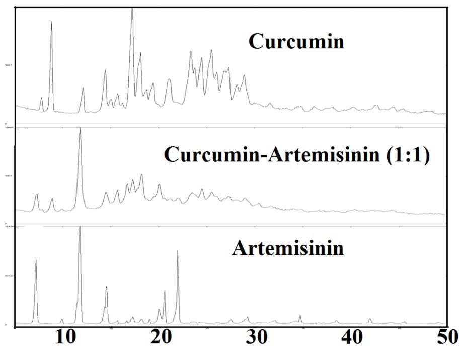
**Figure S1b** Curcumin-Artemisinin (1:1) ball mill grinding PXRD pattern comparison with starting materials.
