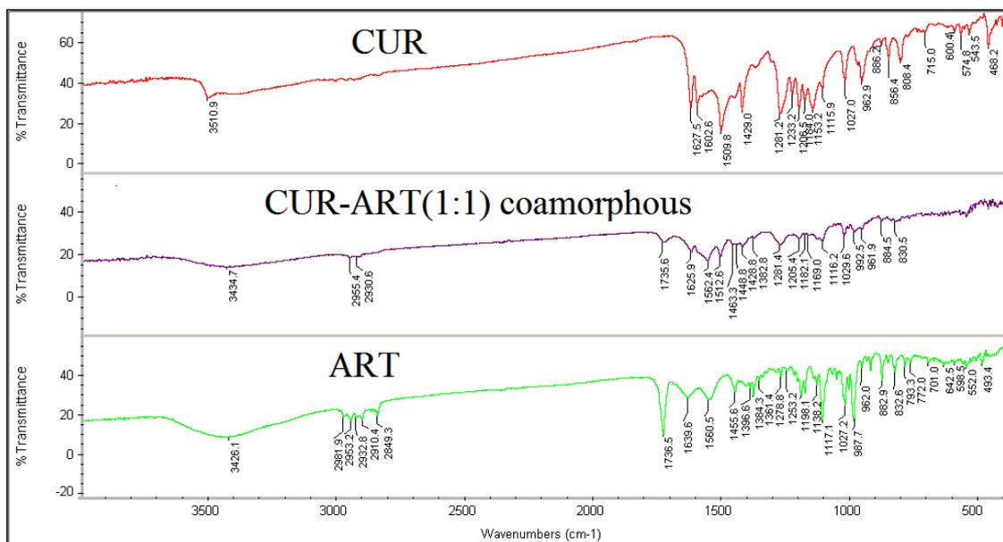
**Figure S6** Overlay of FT-IR spectra of CUR-ART coamorphous compared to the individual components
