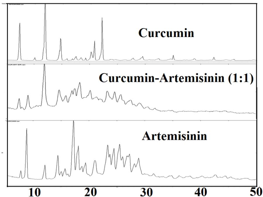
**Figure S9c** PXR D of CUR-ART coamorphous at the end of equilibrium solubility experiment matches with starting materials as a physical mixture of CUR and ART. The material at the end of solubility measurement is more crystalline compared to the grinding product shown in Figure S1 and S2. E.g. there are noticeable peaks after  $2\theta = 20^\circ$ .
