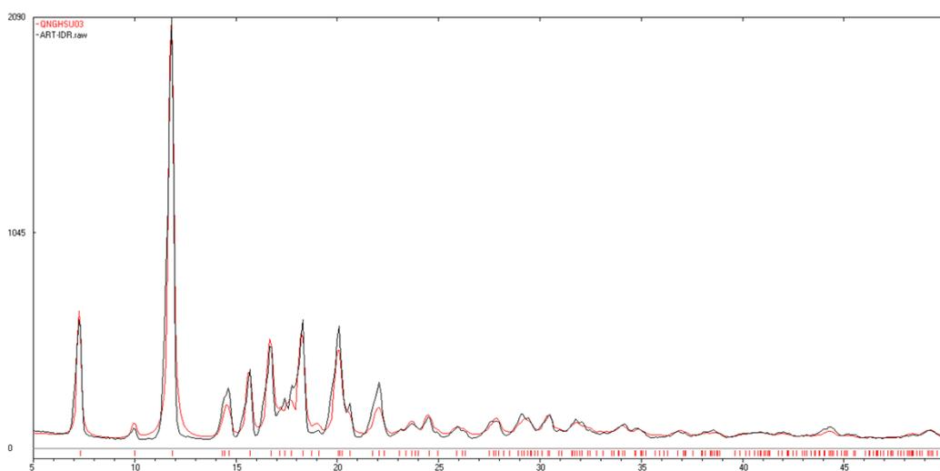
**Figure S9b** PXRD of ART at the end of equilibrium solubility experiment matches with calculated XRD lines of ART form I.
