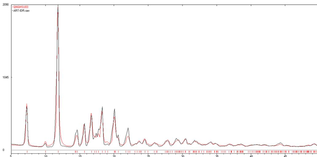
**Figure S9e** PXRD of ART at the end of IDR experiment matches with calculated XRD lines of ART form I.
