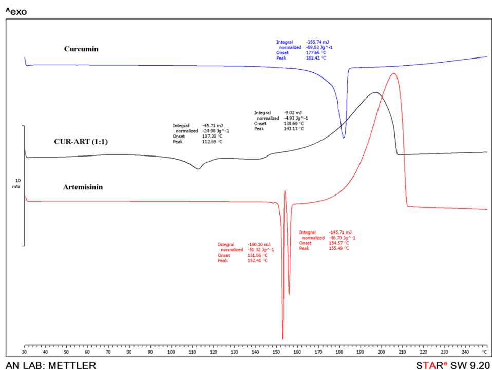
**Figure S2** DSC heating curve of Curcumin-Artemisinin (1:1) (prepared by ball mill grinding) comparison with starting materials.
