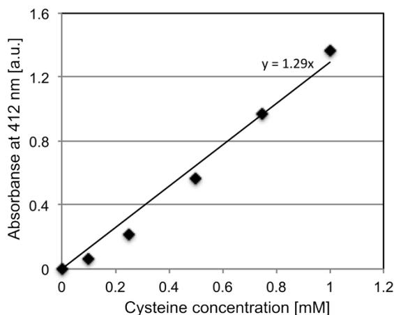
**Figure S1.** A calibration curve obtained by measuring the absorbance of cysteine solution.
