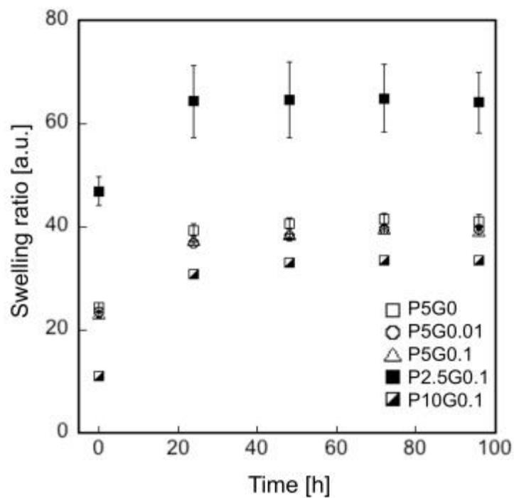
**Figure S2.** Swelling ratio of (PEG-SH)-(Gela-SH) hybrid hydrogels as a function of time. Error bars denote standard deviations (SD) ( $n = 3$ ).
