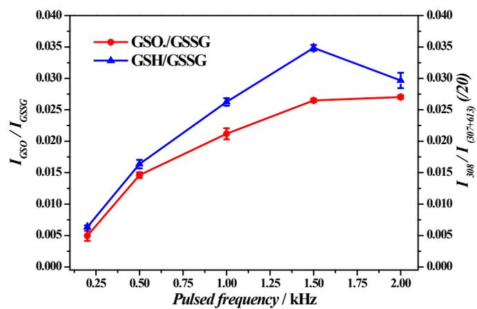
**Fig. S4.** Dependence of DSB dissociation on the frequency of pulsed high voltage (6 kV). In all these experiments,  $\text{NH}_4\text{OAc}$  (5 mM) was added into the spray solution.
