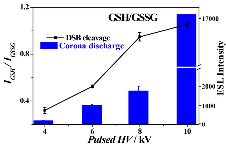
**Fig. S3.** The increase trend of GSH, a pair-product of GSO• from DSB oxidative cleavage, with the increase of amplitude of the pulsed high voltage (1 kHz). Corona discharge and DSB cleavage was observed with a similar increase trend with adjusting of the amplitude of pulsed high voltage.
