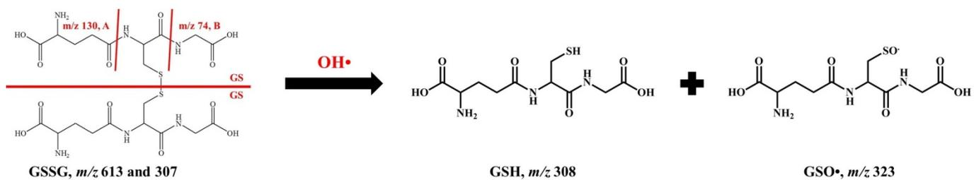
**Scheme S1.** Possible oxidative cleavage reaction pathway for the cleavage of DSB via radical generation in InESI.
