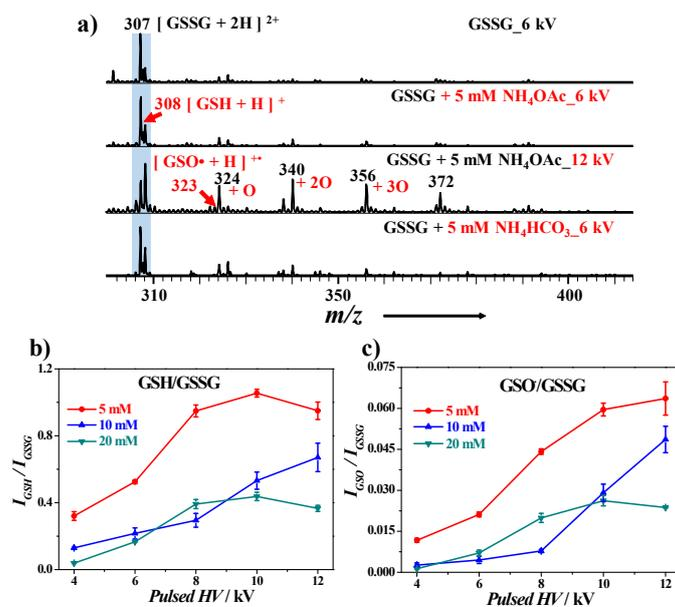
**Fig. S5.** a) Comparison of oxidative cleavage reaction products from GSSG via InESI with different spray voltages and different electrolytes. Dependence of DSB dissociation on low concentration volatile electrolyte and amplitude of pulsed high voltage, as illustrated by b) GSO• and c) GSH. Different concentrations of  $\text{NH}_4\text{OAc}$  were indicated.
