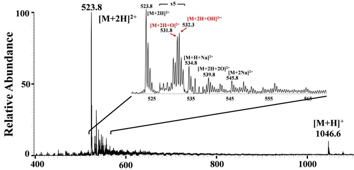
Fig. S1. MS spectrum of the oxidative cleavage products from selectin binding peptide by InESI.
