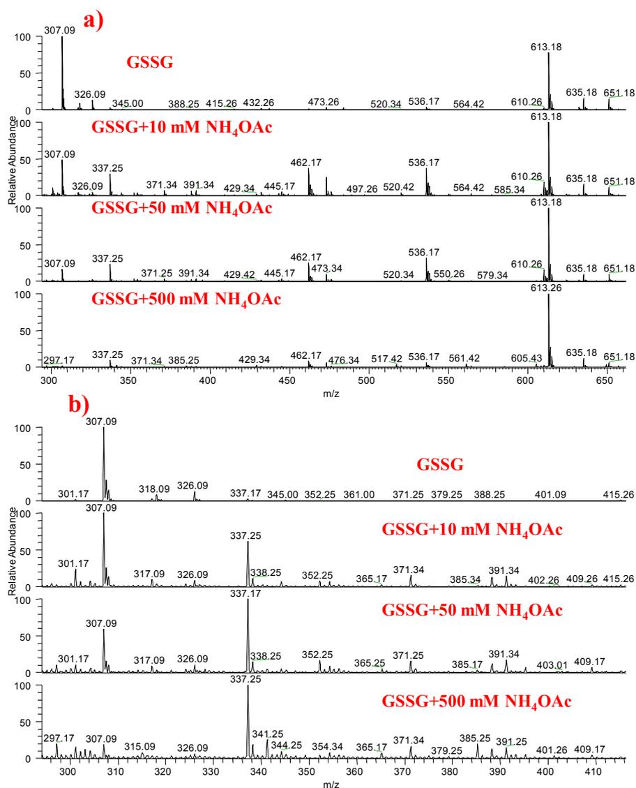
**Fig. S6.** a) Sonic spray ionization MS spectrum of GSSG in the presence of various concentrations of NH<sub>4</sub>OAc. b) Magnification of a) for mass range between m/z 290 and 420. No oxidative cleavage reaction cleavage products (GSH, *m/z* 308 or GSO•, *m/z* 323) were observed in sonic spray ionization for the absence of corona discharge.
