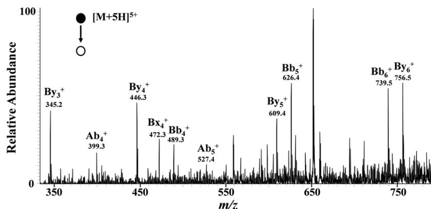
**Fig. S7.** Tandem MS spectrum (low  $m/z$  range) of  $[M+5H]^{5+}$  for human insulin containing 10 mM  $\text{NH}_4\text{OAc}$  derived from “OFF” mode. Sequence information beyond the disulfide bonds were obtained.
