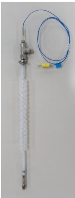
**Fig. S2** A tube reactor
