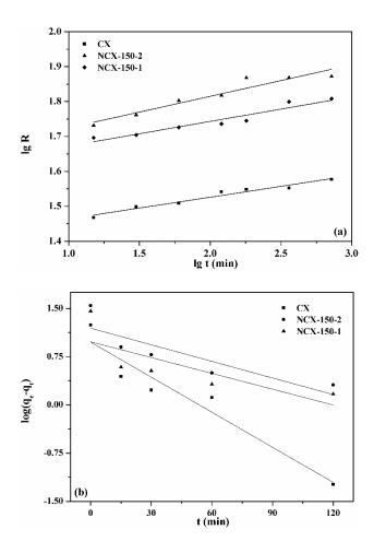
**Figure S1.** The adsorption kinetics including (a) intraparticle diffusion and (b) pseudo-first-order models.
