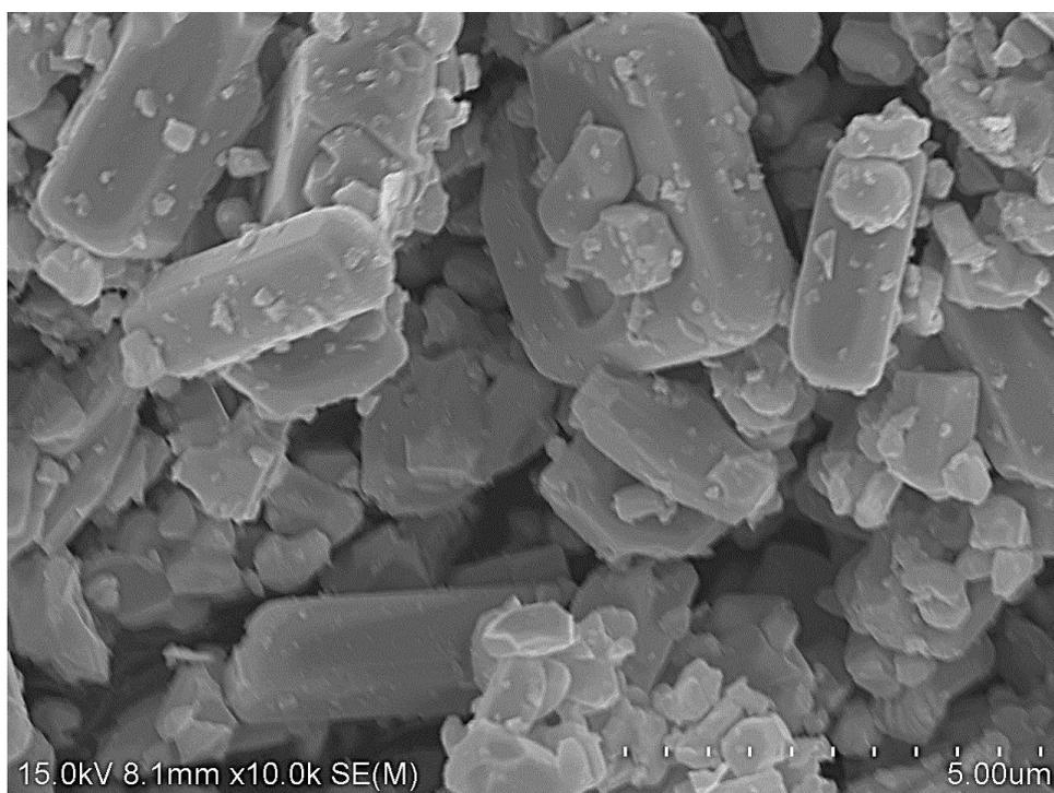
Fig.S7 SEM image of commercial  $\text{Cs}_{0.33}\text{WO}_3$  obtained from Sumitomo Metal Mining Co., Ltd, Japan.
