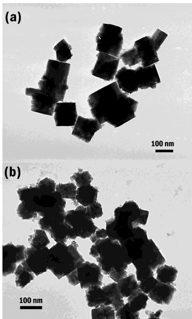
Fig.S6 TEM image of sample synthesized after (a) 0.5 and (b) 2 h reaction
