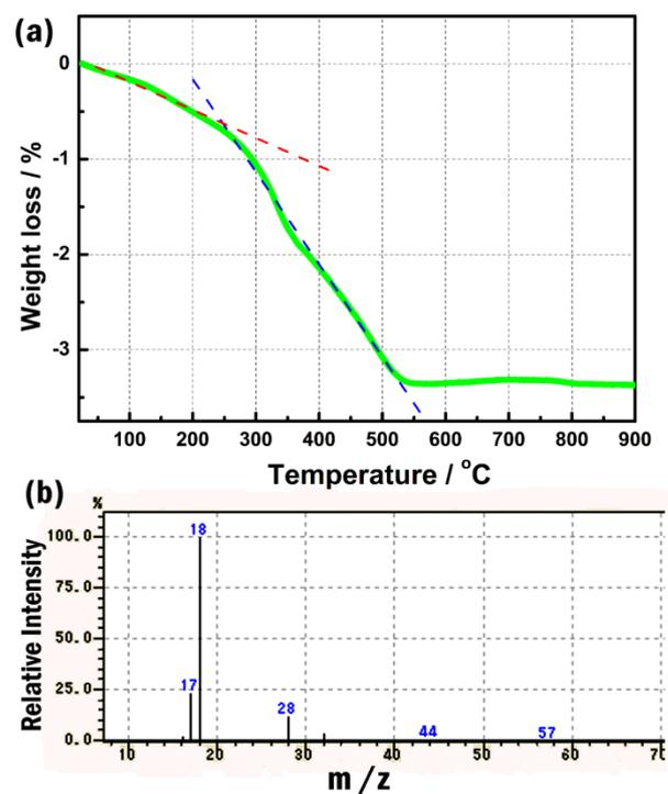
**Fig. S3** (a) TG curve recorded at a heating rate of 10 °C/min and (b) MS results for the gas produced during the heating.
