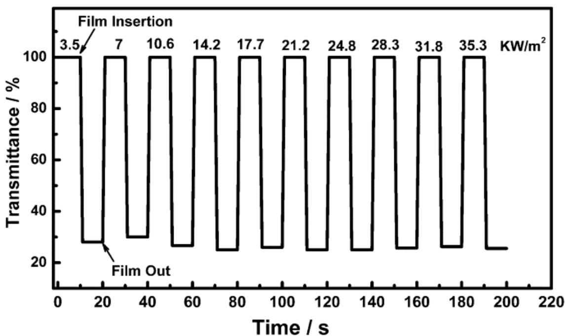
**Fig. S9** The transmittance spectra of  $(\text{NH}_4)_x\text{WO}_3$  film irradiated by varied powder density ( $3.5 - 35.3 \times 10^5 \text{ W}\cdot\text{m}^{-2}$ ) of 1064 nm light. The  $(\text{NH}_4)_x\text{WO}_3$  film was set on the light path for 10s and then taken out, alternately.
