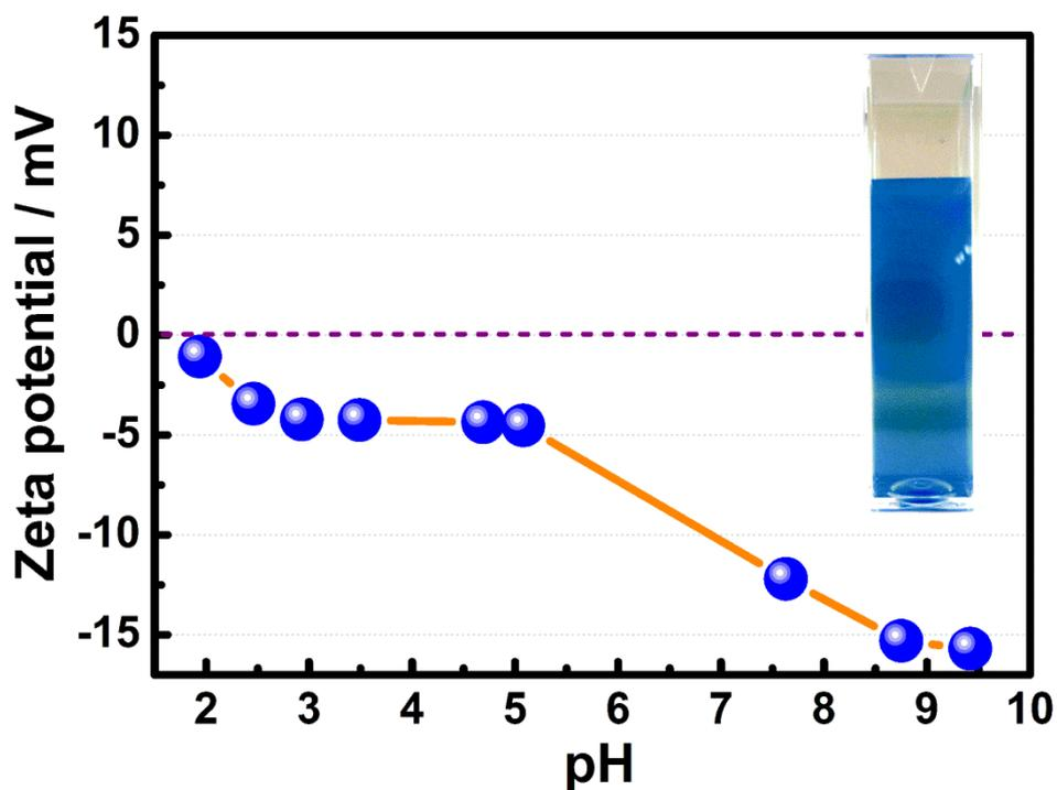
Fig.S9 Zeta potential versus pH for  $(\text{NH}_4)_x\text{WO}_3$  nanocube. Inset shows the suspension of  $(\text{NH}_4)_x\text{WO}_3$  nanocube.
