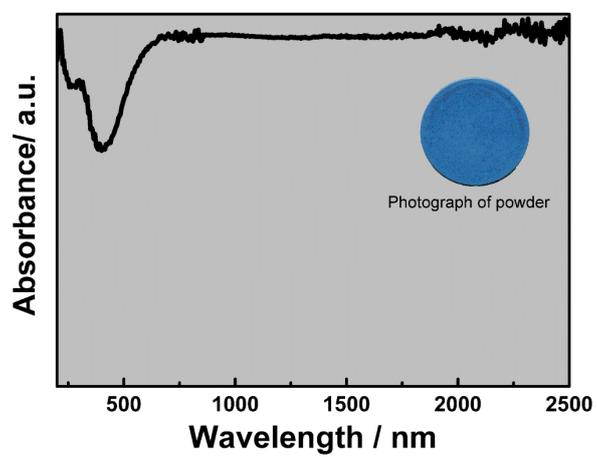
**Fig.S8** Absorbance spectra of  $(\text{NH}_4)_x\text{WO}_3$  nanocubes; Inset shows the photograph of blue powder
