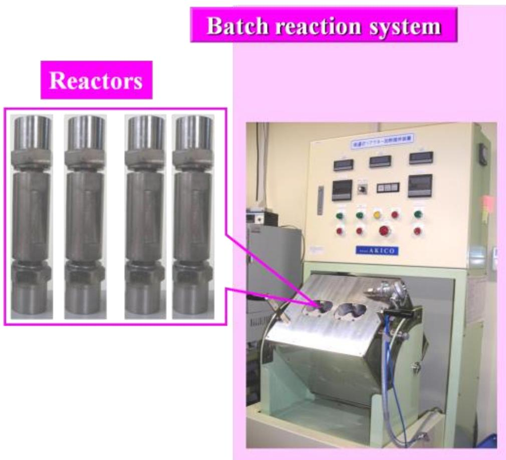
**Figure S1** Batch reaction system (Akico Co. Ltd., Japan) and reactors.
