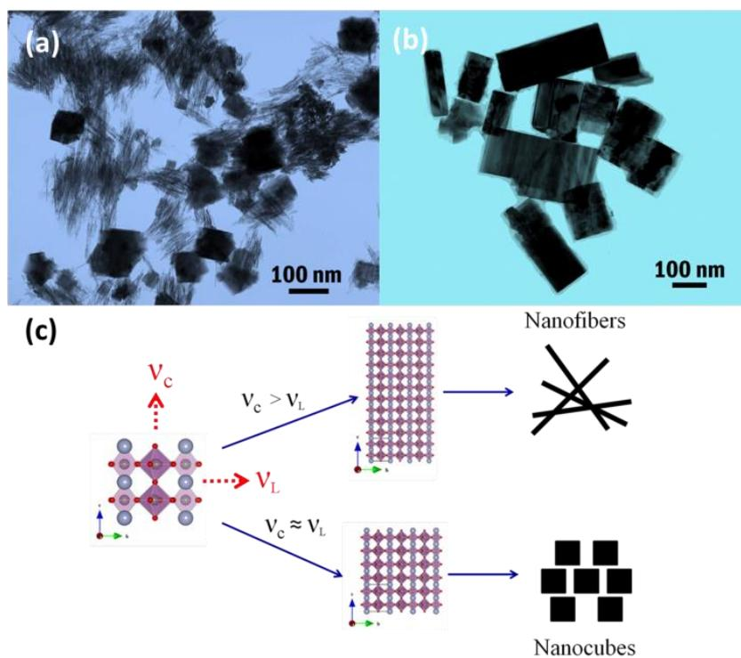
**Figure S4** TEM images of samples synthesized with addition of (a) 1 ml or (b) 5 ml oleylamine, while keeping other parameters the same to the standard conditions; (c) proposed crystal growth process for the formation of tungsten bronzes in the presence or absence of the capping agent.
