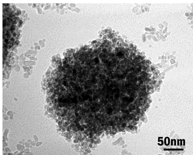
**Fig.S5** (a) XRD pattern and (b) TEM image of sample synthesized in pure oleic acid solution
