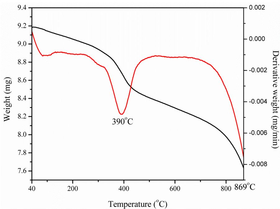
Figure S1 TGA-DTA curve of ZBO 2
