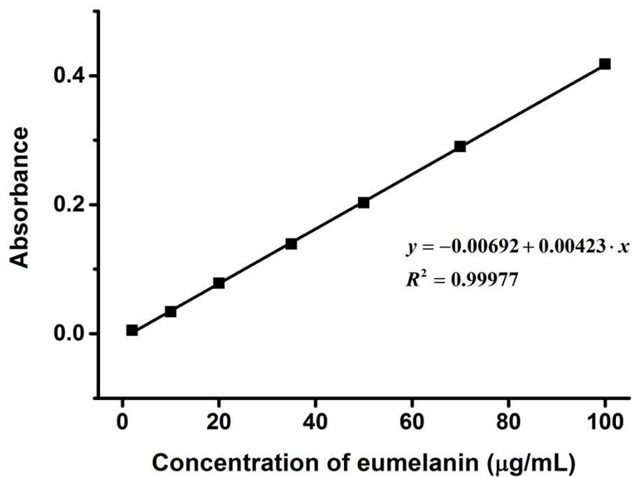
**Figure S2** Eumelanin concentration was determined using optical density at 400 nm. The calibration curve was prepared by measuring absorbance of commercial eumelanin in M9 at different concentrations: 2, 10, 20, 35, 50, 70, 100 µg/mL.
