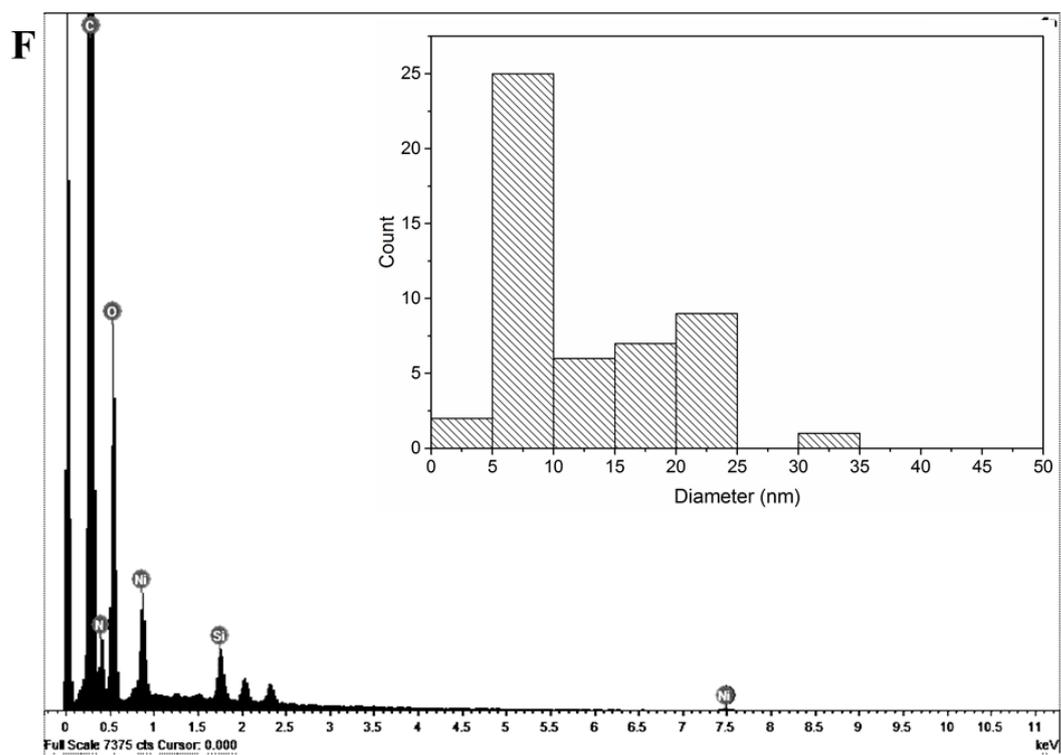
**Figure S4** EDS spectra show the presence of (A) Au in Figure 2A, (B) Ag in Figure 2B, (C) Cu in Figure 2C, (D) Mn in Figure 2D, (E) Pt in Figure 2E, (F) Ni in Figure 2F. Inset: Histograms of size distribution of metal nanoparticles from corresponding TEM images.
