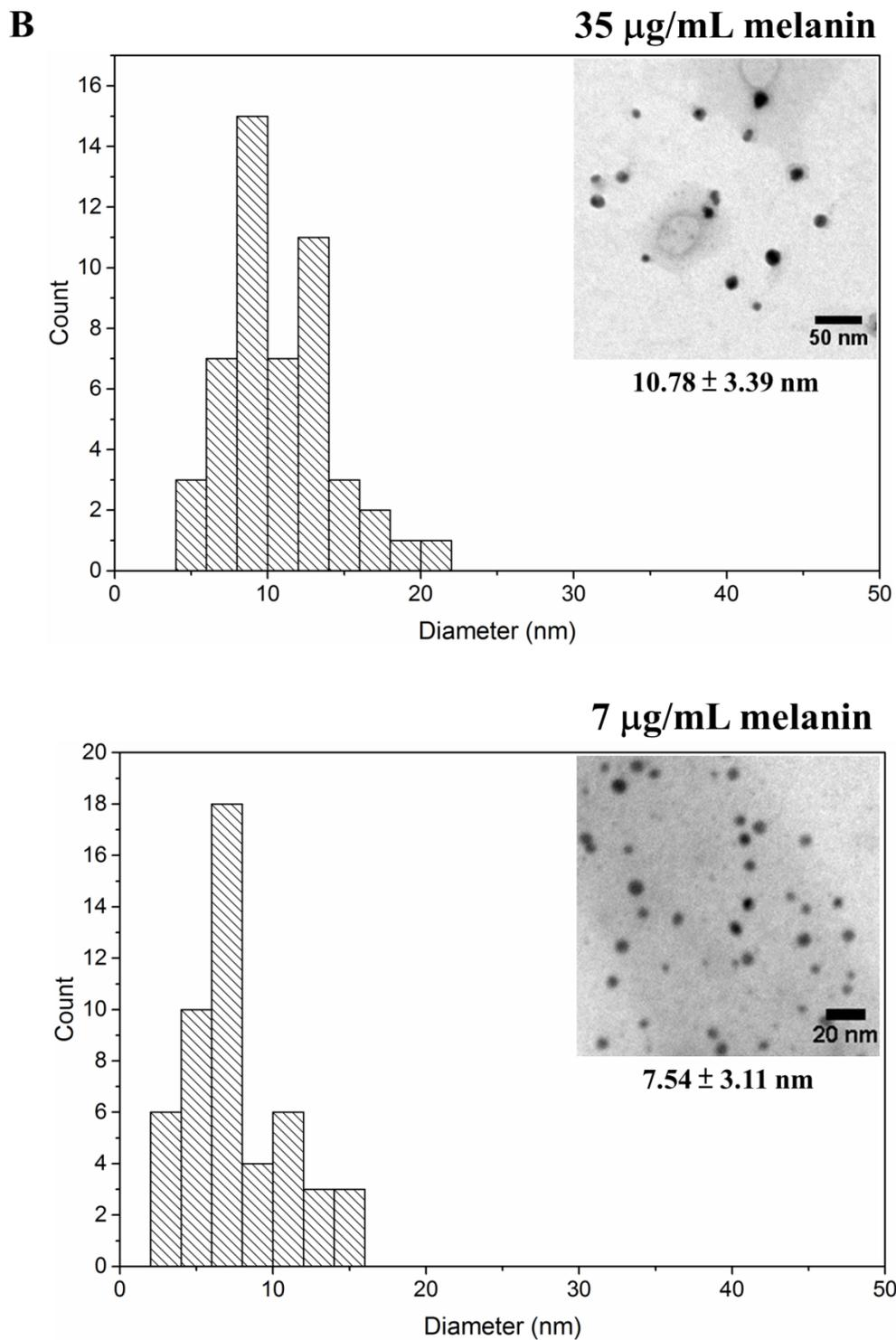
**Figure S5** Histograms of size distribution analysis of Au nanoparticles from corresponding TEM images (A) at the different concentrations of  $\text{Au}^{3+}$  (B) at the different concentrations of eumelanin.
