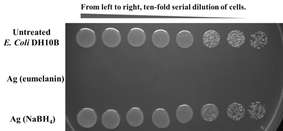
**Figure S6** Growth and comparison of various metal nanoparticles treated cells. Quantitative survival measurements of *E. coli* DH10B in the presence or absence of 150 $\mu$ g/mL of Ag nanoparticles prepared by EuMel or NaBH<sub>4</sub>.
