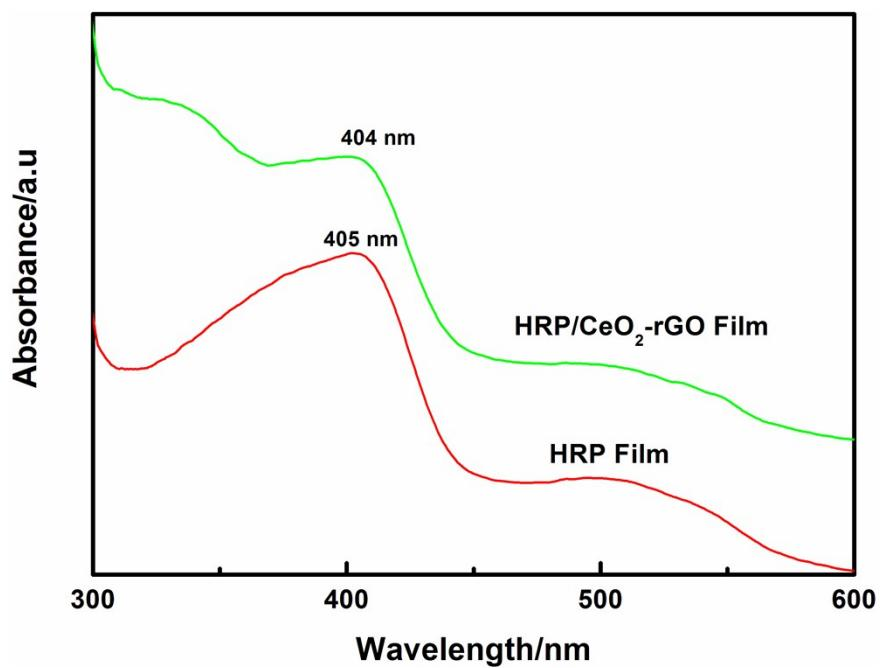
Fig. S2 UV-vis spectra of HRP and HRP/CeO<sub>2</sub>-rGO film on quartz slides at room temperature.
