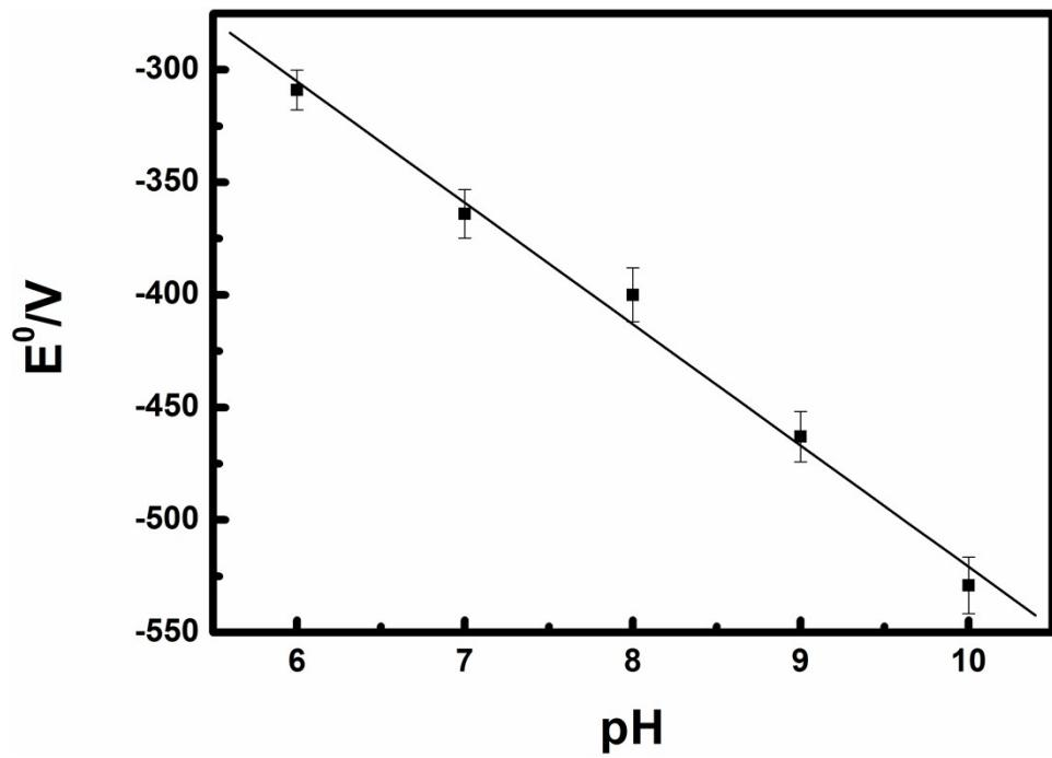
**Fig. S4** Plot of formal potential *vs.* pH for HRP/CeO<sub>2</sub>-rGO modified GC electrodes in 0.1 M PB solution (pH 7.0) at scan rate 100 mV/s.
