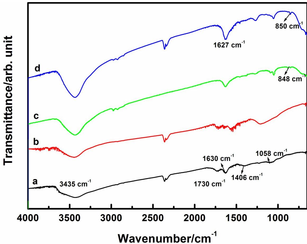
**Fig. S1** FT-IR spectra of (a) GO, (b) rGO, (c) CeO<sub>2</sub>-rGO and (d) CeO<sub>2</sub>.
