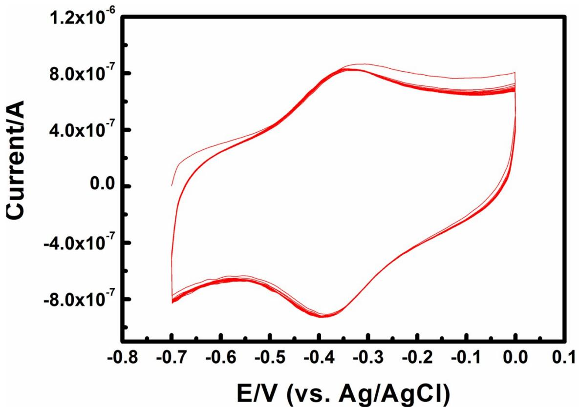
**Fig. S5** CVs stability of HRP/CeO<sub>2</sub>-rGO modified GC electrode in PB solution (pH 7.0) at a scan rate of 100 mV/s for 20 continuous cycles in the potential window between -0.7 to 0 V.
