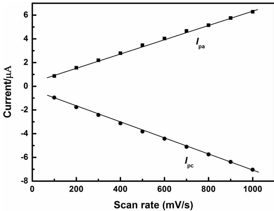
**Fig. S3** Plot of peak current as a function of scan rates for HRP/CeO<sub>2</sub>-rGO modified GC electrode in PB solution (pH 7.0).
