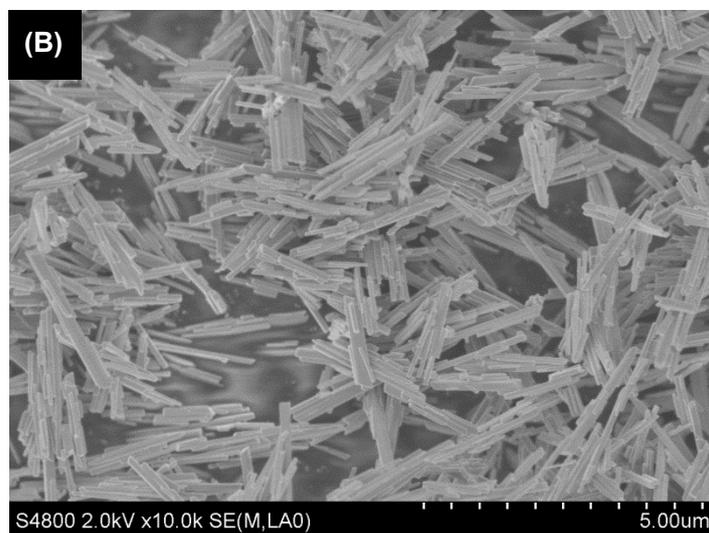
**Figure S1.** (A) X-ray diffraction pattern and (B) scanning electron microscopy image of PbCrO<sub>4</sub> particles prepared by simple precipitation method.
