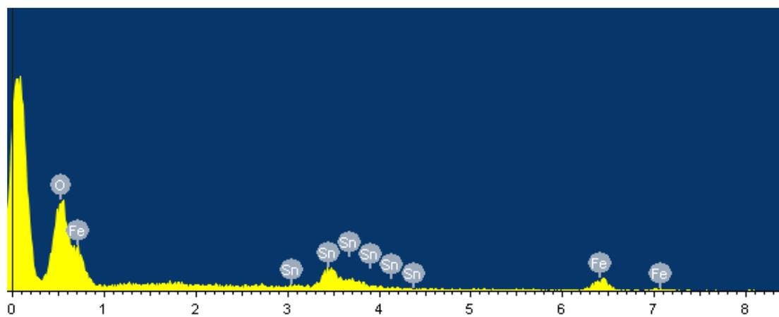
**Figure S3.** EDS spectrum of Sn:Fe<sub>2</sub>O<sub>3</sub> film.
