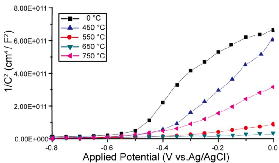
**Figure S2.** Mott-Schottky plots under dark condition at a frequency of 1 KHz for different annealing temperature of the samples.
