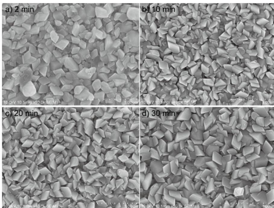
**Figure S4** SEM images of different doping levels, and this parameter depended on laser ablation duration.
