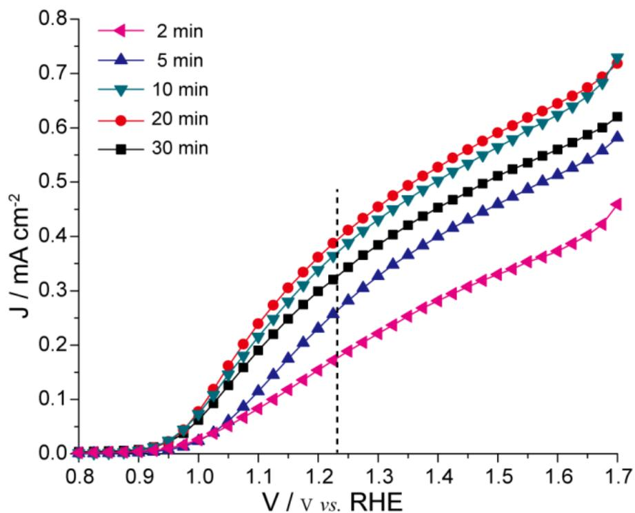
**Figure S5.**  $J$ - $V$  curves of different Sn doping concentrations (after thermal treatment at  $600^{\circ}\text{C}$ ). Sn doping levels were tuned by adjusting the concentrations of the Sn colloidal solution, and this parameter depended on the duration time of laser ablation.
