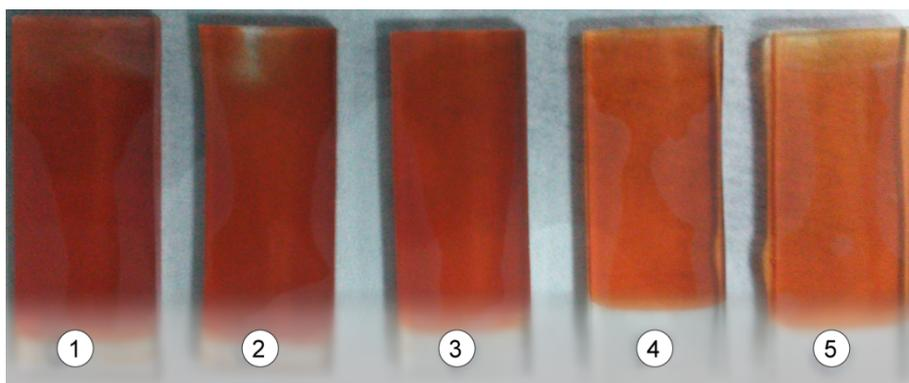
**Figure S6.** Photo-images of hematite nanocrystalline films with different Sn-doped concentration. Different ablation duration for Sn colloidal solutions: (1) 2 min, (2) 5 min, (3) 10 min, (4) 20min, (5) 30min.
