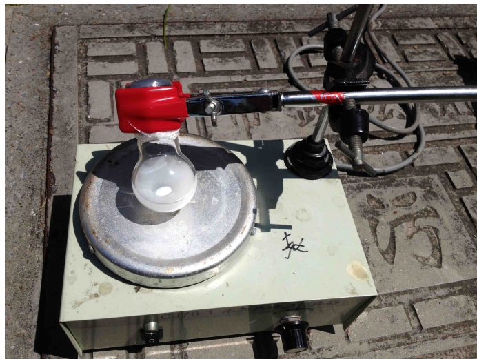
Fig. S2 The photo of outdoor equipment of sunlight-driven water splitting by ZnO/ZnS system in Wuxi city 2014. Experimental condition: Outdoor temperature: 30 ~ 32 °C, Time: 10: 00 ~ 14: 00.
