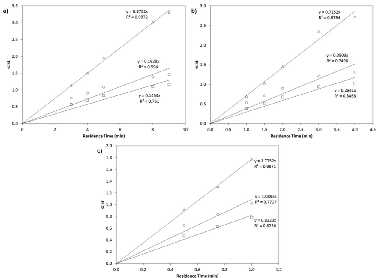
**Figure S5.** Application of different kinetic models to the experimental data of the Petasis reaction of salicylaldehyde at a) 160 °C, b) 180 °C, and c) 200 °C. Y-axis is proportional to  $kt$  resulting from each kinetic model: first-order (○), second-order non-equimolar (□), second-order equimolar (△) rate-limiting step.
