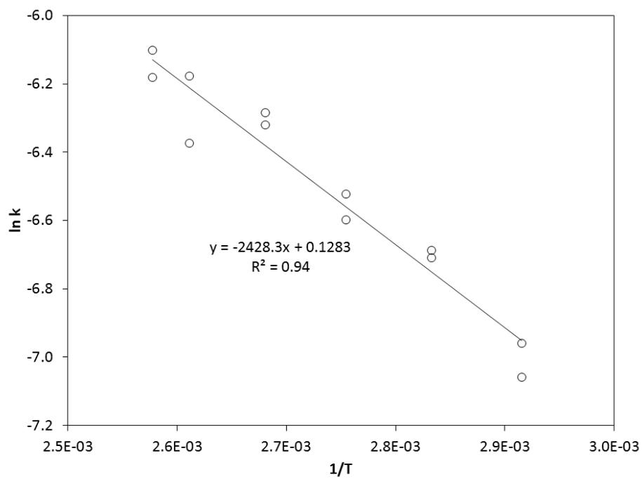
**Figure S7.** Arrhenius plot of  $\ln k$  (L/mol·s) versus  $1/T$  (K<sup>-1</sup>) for the Ugi reaction employing the Petasis product as a reactant.
