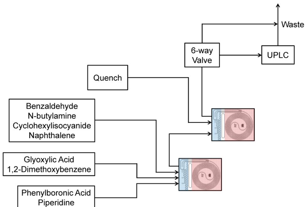
**Figure S3.** Setup of the microreactor system employed to study the Petasis-Ugi tandem reaction.
