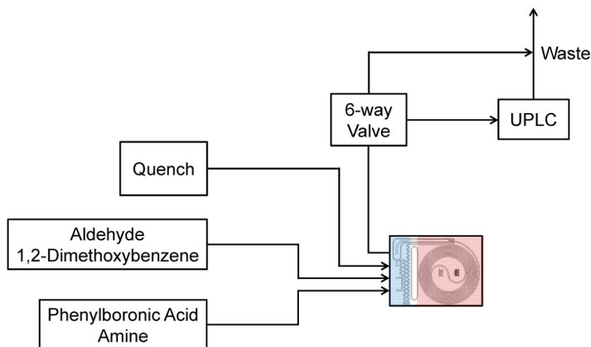
**Figure S2.** Setup of the microreactor system employed to study the Petasis reaction.
