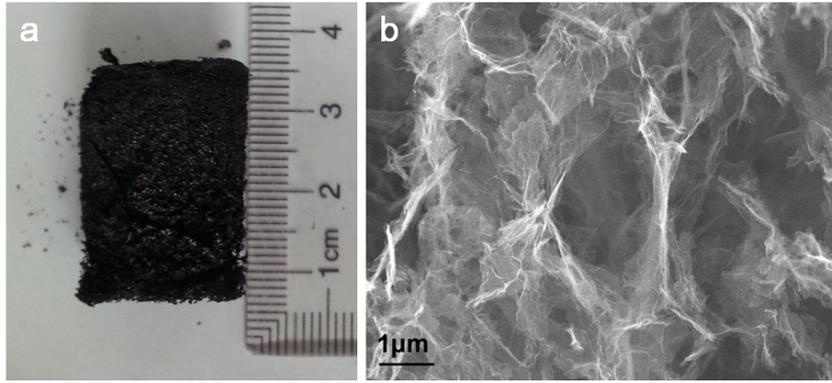
Figure S1. (a) Optical image of OMC/GA and (b) SEM image of GA
