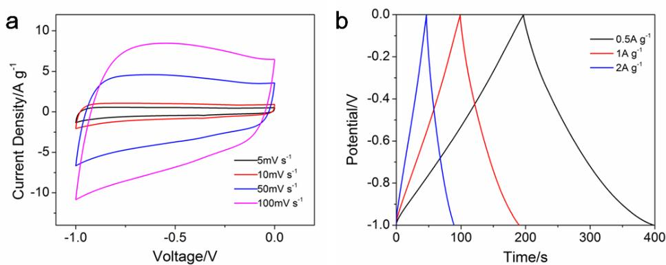
Figure S4. (a) CVs and (b) galvanostatic charging/discharging curves of the GA.
