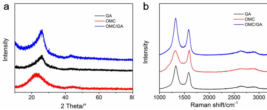
Figure S3. (a) XRD patterns and (b) Raman spectra of OMC/GA, GA and OMC
