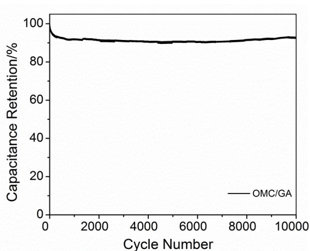
Figure S5. Cycling stability of OMC/GA electrodes.
