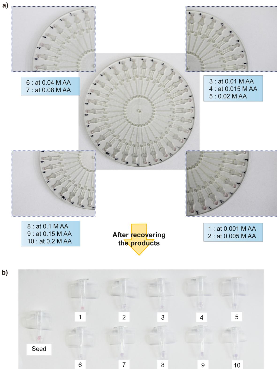
**Figure S2** a) Digital images of the microreactors in which the gold nanoparticles were synthesized at different concentrations of ascorbic acid (AA), b) Digital images of the recovered Au NP products in a 0.2 mL PCR tube. The color of the Au NPs changed from pink to blue-purple as the concentration of AA increased.
