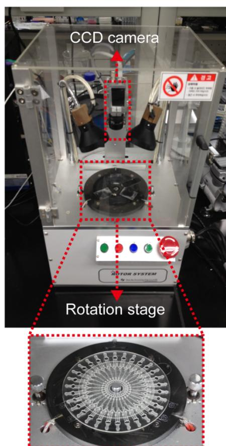
**Figure S1** Digital images of the rotary stage and the rotary microfluidic device.
