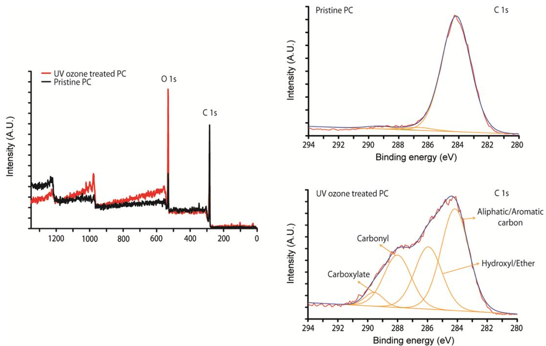
**Figure S3** XPS data before and after the UV ozone treatment on the PC layer.
