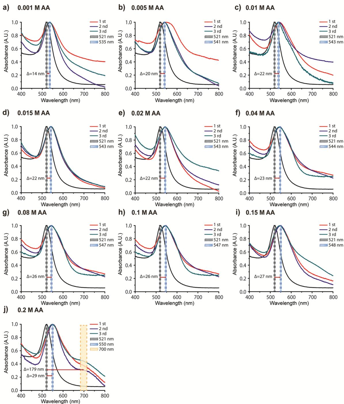
**Figure S4** UV-Vis absorption spectra of the triplicate Au NPs synthesized at different concentrations of ascorbic acid: a) at 0.001 M, b) 0.005 M, c) 0.01 M, d) 0.015 M, e) 0.02 M, f) 0.04 M, g) 0.08 M, h) 0.1 M, i) 0.15M, and j) 0.2 M.
