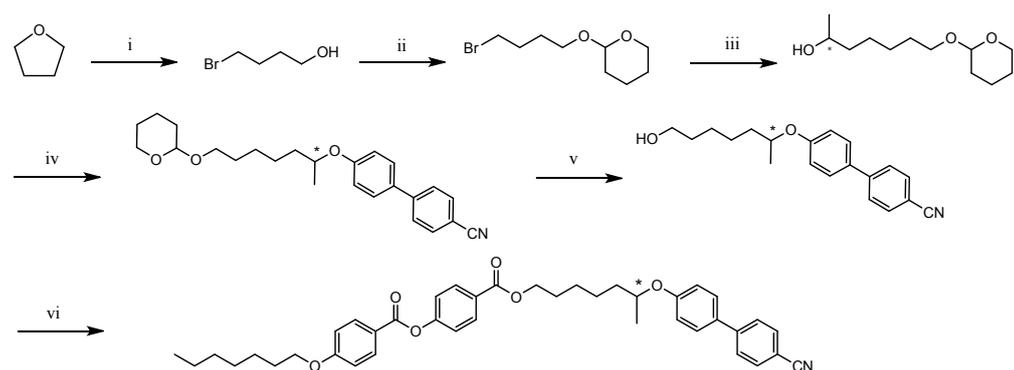
Reagents and conditions: (i) HBr (48% in water), THF, reflux, 4 h; (ii) PPTS, DCM, r.t., (iii) Mg, (R)-(+)-Propylene oxide, THF, CuI, (iv) 4'-hydroxy-[1,1'-biphenyl]-4-carbonitrile, DIAD, PPh<sub>3</sub>, THF, 0 °C, 15 min, then r.t., overnight (v) TsOH, MeOH, CH<sub>2</sub>Cl<sub>2</sub>, refluxed (vi) 4-((4-(heptyloxy)benzoyl)oxy)benzoic acid, DCC, DMAP, DCM, r.t., overnight.
