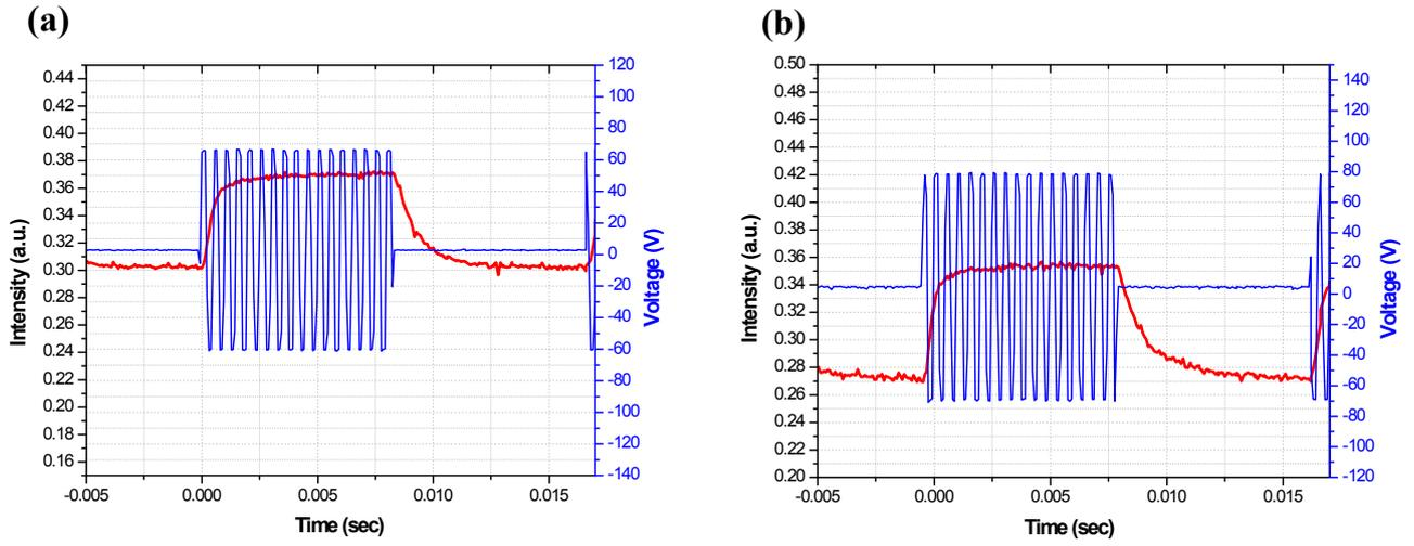
**Figure S3.** Diads **II-B** and **III-D** in BPs at  $T-T_{LBP} = -2^{\circ}\text{C}$ . (a) Electro-optical response curves of **II-B** at  $13 \text{ V}\mu\text{m}^{-1}$ . (b) Electro-optical response curves of **III-D** at  $15 \text{ V}\mu\text{m}^{-1}$ .
