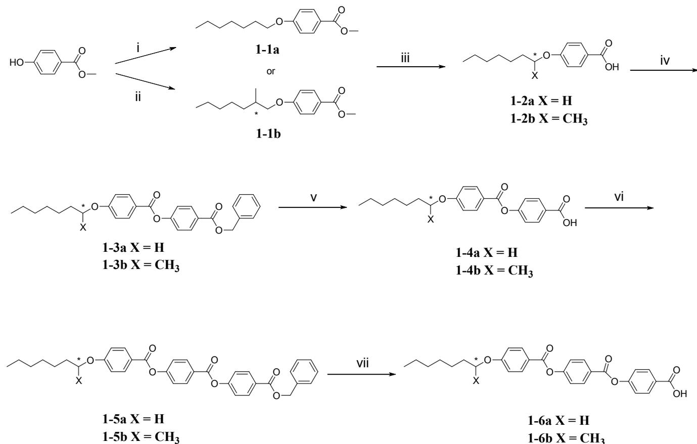
Reagents and conditions: (i) 1-bromoheptane, K<sub>2</sub>CO<sub>3</sub>, KI, acetone, reflux, 24 h; (ii) (S)-(+)-2-octanol, DIAD, PPh<sub>3</sub>, THF, 0 °C, 15 min, then r.t., overnight; (iii) KOH, MeOH, reflux, overnight, then HCl aqueous; (iv) benzyl 4-hydroxybenzoate, DCC, DMAP, DCM, r.t., overnight; (v) H<sub>2</sub>, 10% Pd-C, THF, r.t., 10 h; (vi) benzyl 4-hydroxybenzoate, DCC, DMAP, DCM, r.t., overnight; (vii) H<sub>2</sub>, 10% Pd-C, THF, r.t., 10 h.
