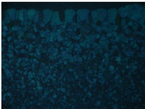
**Figure S1.** POM texture of **III-B** at 181.0 °C upon cooling (0.5 °Cmin<sup>-1</sup>).
