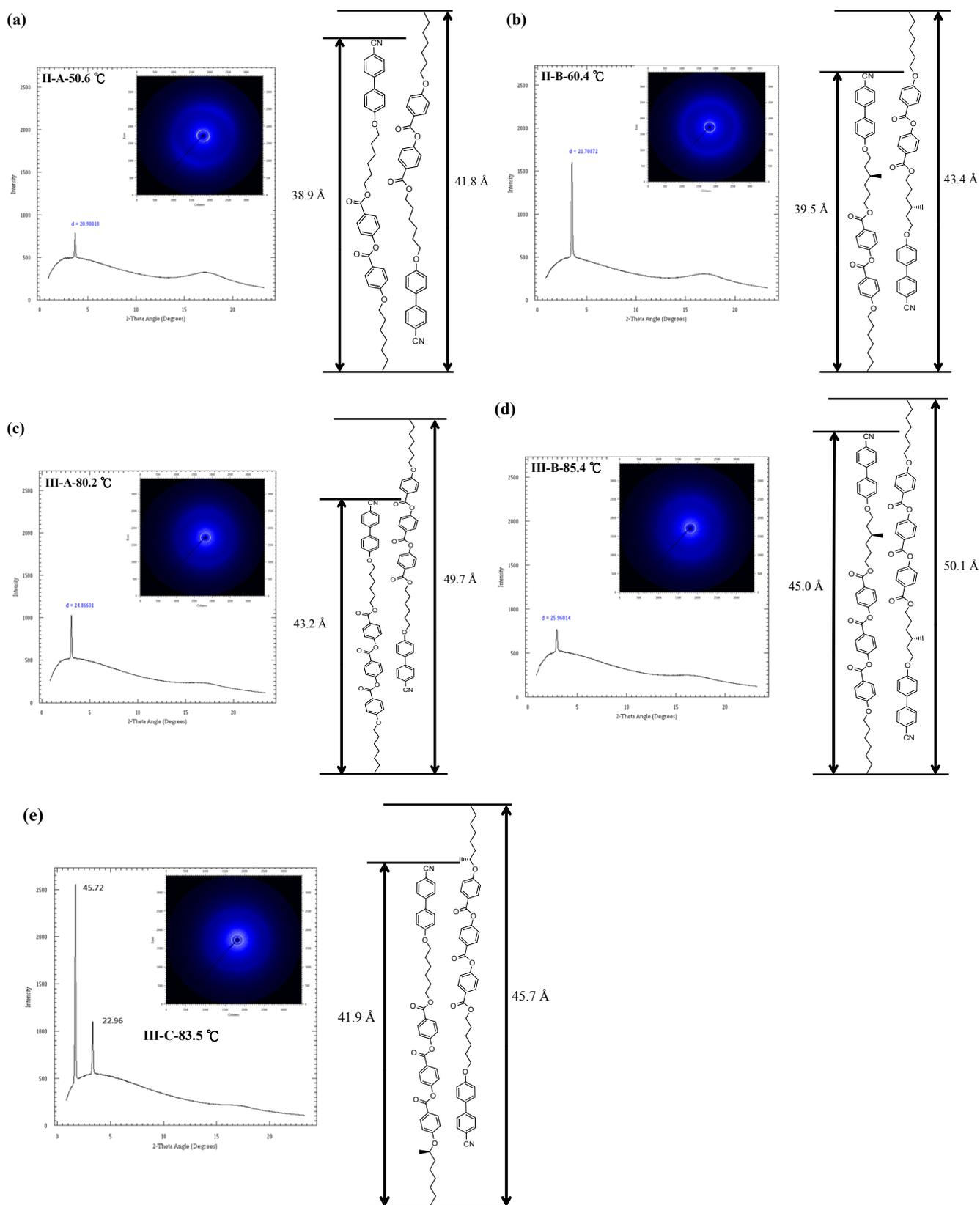
**Figure S2.** Powder XRD Analyses of (a) **II-A** at 50.6 °C, (b) **II-B** at 60.4 °C, (c) **III-A** at 80.2 °C, (d) **III-B** at 85.4 °C and (e) **III-C** at 83.5 °C.
