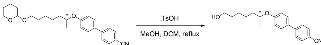
To a stirred solution of **3-4** (1.0 g, 2.54 mmol) and TsOH (0.1 g, 0.53 mmol) was dissolved in MeOH (20 ml) and CH<sub>2</sub>Cl<sub>2</sub> (20 ml). The mixture was refluxed and stirred for 10 h. The resulting mixture was poured into water and extracted with dichloromethane. The organic layer was dried over Na<sub>2</sub>SO<sub>4</sub> and evaporated to afford compound **3-5** as a light white solid in 85 % yield.
