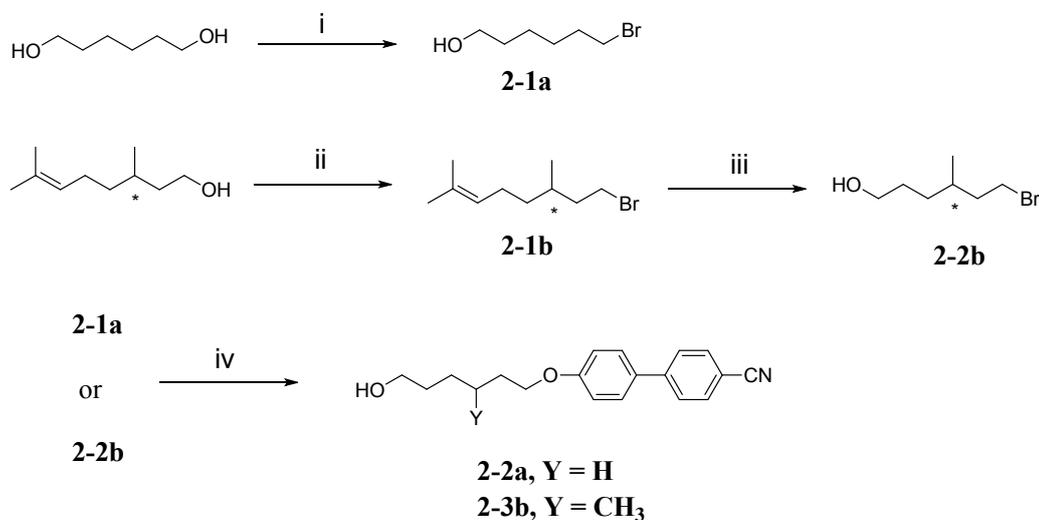
Reagents and conditions: (i) HBr (48% in water), toluene, reflux, 18 h; (ii) CBr<sub>4</sub>, PPh<sub>3</sub>, DCM, 0°C, then, r.t. 2 h; (iii) O<sub>3</sub>, MeOH, -78 °C, 2h, after NaBH<sub>4</sub>, MeOH, r.t., overnight, then water, H<sub>2</sub>SO<sub>4</sub>, (iv) 4'-hydroxy-4-biphenylcarbonitrile, K<sub>2</sub>CO<sub>3</sub>, KI, acetone, reflux, 24 h.
