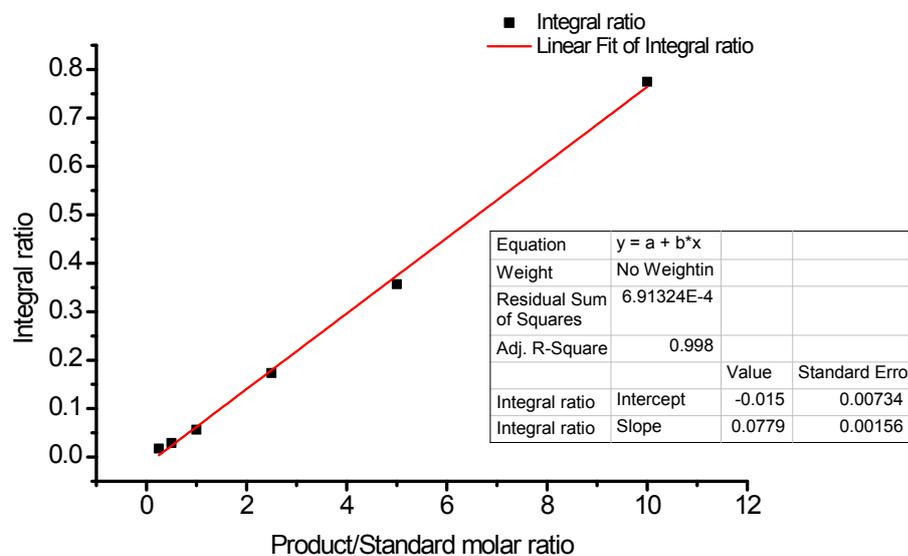
**Figure S2.** Calibration curve based on  $^1\text{H}$  NMR analysis (in  $d_6$ -acetone) for the yield calculation for Suzuki-Miyaura coupling reaction (product is biphenyl-4-carboxylic acid; standard is hexadecane).
