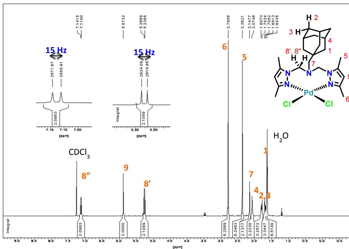
**Figure S1.** (top) <sup>1</sup>H NMR spectrum of the ligand Ad-L in CDCl<sub>3</sub> (300 MHz, 25 °C); (bottom) <sup>1</sup>H NMR spectrum of the Pd(II) complex Ad-L-PdCl<sub>2</sub> in CDCl<sub>3</sub> (500 MHz, 25 °C).
