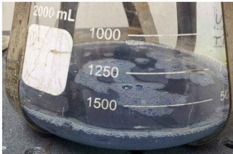
Figure S1. The CYP101B1 E. coli whole-cell oxidation system after the addition of indole.
